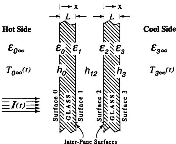
Figure 1. Double-Pane Geometry Showing the Numbering System and the Inter-Pane Gap.
