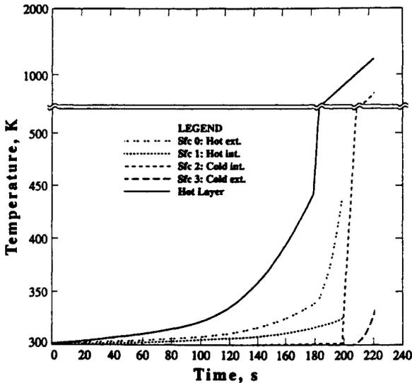
Figure 5. McBreak Double-Pane Results Using Default BREAK1 Input Data Values. All input parameters are the same as in Figure 4 except  $l(t)=0$ .
