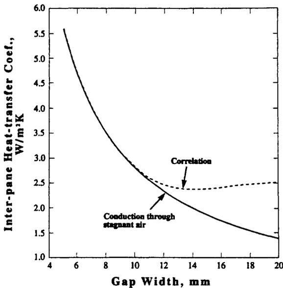
Figure 2. Inter-Pane Heat-Transfer Coefficient,  $h_{12}$ , with the Inter-Pane Gas as Air at  $325\text{K}$  and  $T_1 - T_2 = 50\text{K}$ . The solid line is stagnant conduction and the dashed line the Rayleigh no. correlation,<sup>22</sup>  $Nu[1 + (0.0303Ra^{0.402})^{11}]^{1/11}$ . For argon as the gap gas, lower  $h$  by a factor of approximately  $2/3$ .
