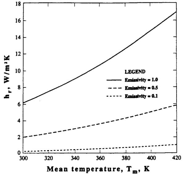
Figure 3. Linearized Heat-Transfer Coefficient,  $h_r$ , as a Function of Mean Temperature,  $T_m$ , where
