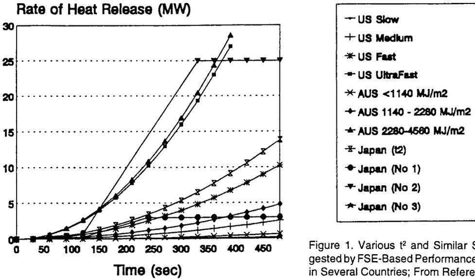
Figure 1. Various  $t^2$  and Similar Simplified Fires, as Suggested by FSE-Based Performance Codes Being Developed in Several Countries; From Reference 1.
