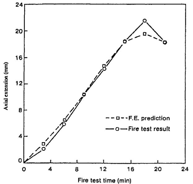
Figure 3. Behavior of a Steel Column under Fire Condition.
