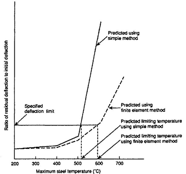
Figure 11. Inaccuracy of Predicted Limiting Temperature Using Simple Method.
