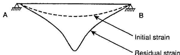
Figure 5. Distribution of Strain in Beam.
