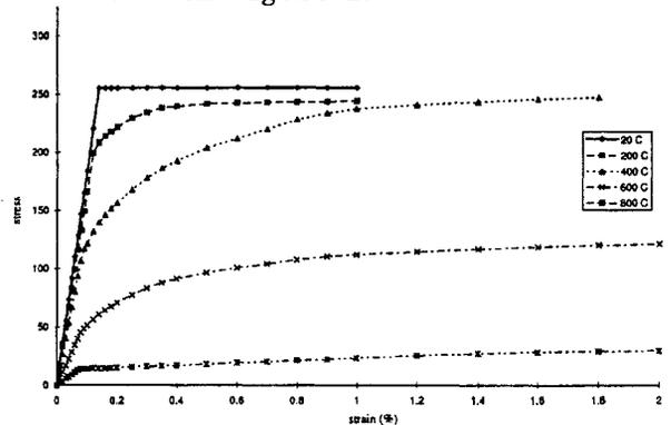
Figure 1. Steel Stress-Strain Curves at High Temperatures, Yield Stress = 255 MPa.
