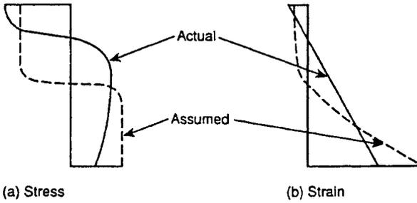
Figure 6. Distribution of Stress and Strain in Steel.
