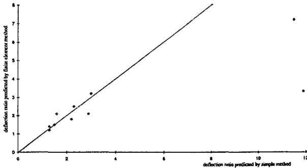
Figure 10. Correlation between Predictions from Finite Element Method and Simple Method.
