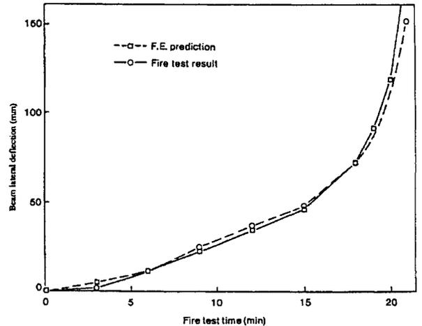
Figure 2. Behavior of a Simply Supported Steel Beam under Fire Condition.
