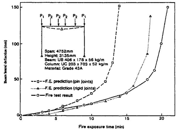
Figure 4. Behavior of a Steel Portal Frame under Fire Condition.
