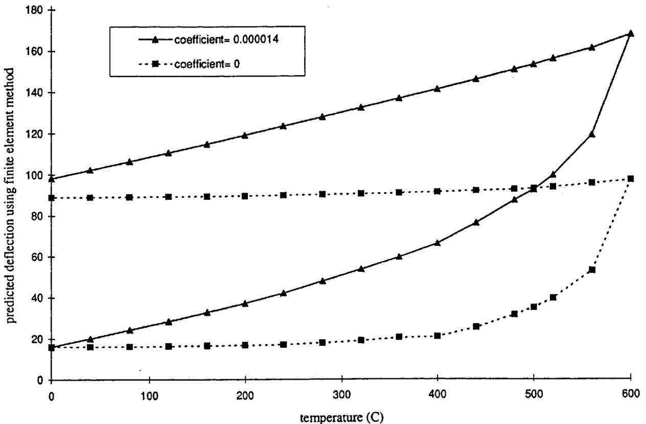
Figure 9. Deflection Curves for Two Values of Coefficient of Thermal Expansion of Steel.
