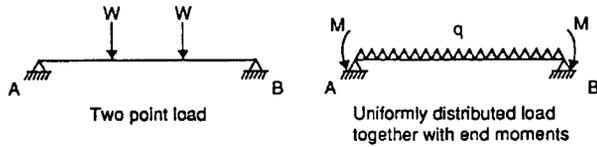
Figure 7. Two Types of Load Distribution.
