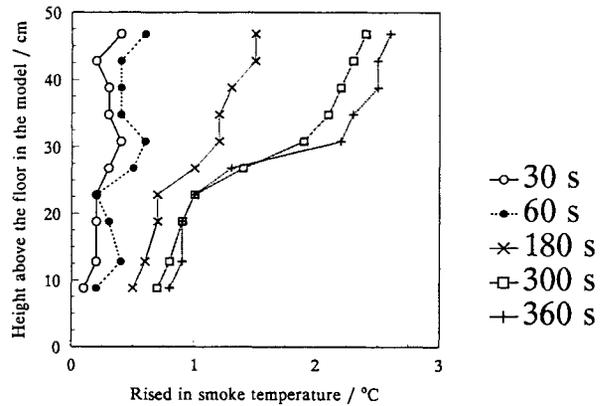
Figure 8. Vertical Distribution of Smoke Layer Temperature Rised in the Atrium for Test 1-1.
