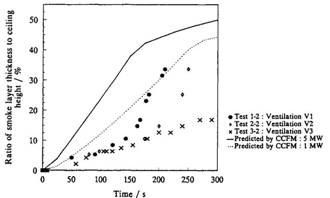
Figure 6. Development of the Smoke Layer in the Atrium Space for a Fire at the Shopping Mall Level 2.
