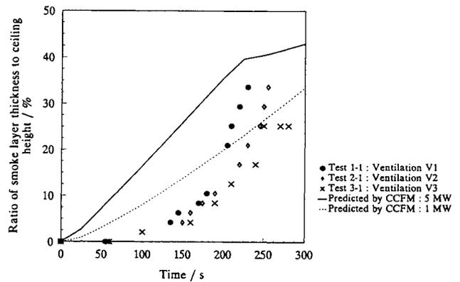
Figure 5. Development of the Smoke Layer in the Atrium Space for a Fire at the Shopping Mall Level 1.
