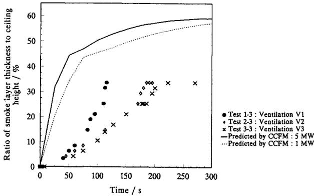
Figure 7. Development of the Smoke Layer in the Atrium Space for a Fire at the Centre of the Atrium Space.
