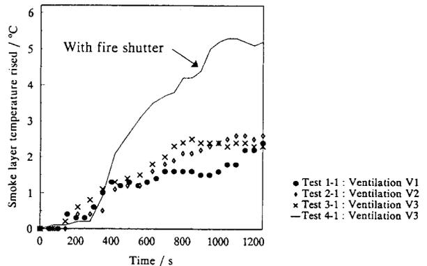
Figure 9. Smoke Layer Temperature Rised in the Atrium Space for a Fire at the Shopping Mall Level 1.
