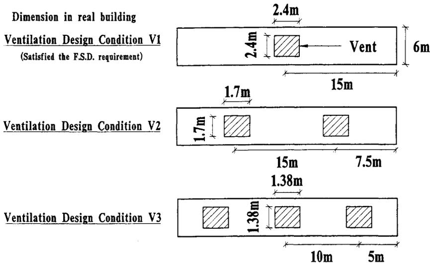
Figure 2. Plan of the Roof Showing the Three Ventilation Conditions.
