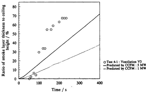
Figure 10. Development of the Smoke Layer in the Atrium Space for a Fire at the Shopping Mall Level 1 with Fire Shutter Operated.
