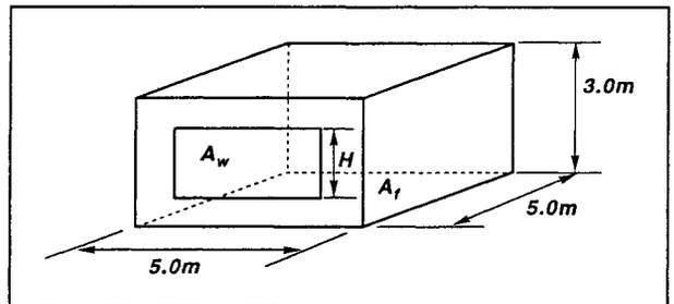
Figure 5. Layout of Compartment Used in COMPF-2 Model.
