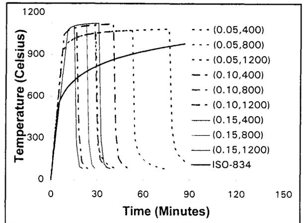
Figure 7. Families of Time Temperature Curves Input to TASEF.
