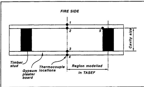
Figure 1. Positions in Test Wall Referred to in Text.
