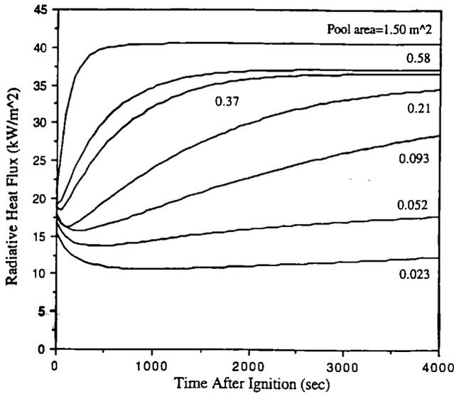
Figure 6. Computed flame radiative heat flux for seven square PMMA pool fires.
