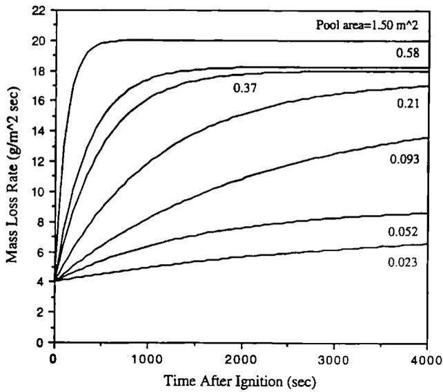
Figure 4. Experimental burning rate for seven square PMMA pool fires<sup>9</sup>.
