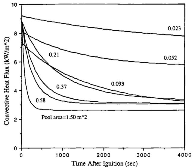
Figure 5. Computed flame convective heat flux for seven square PMMA pool fires.
