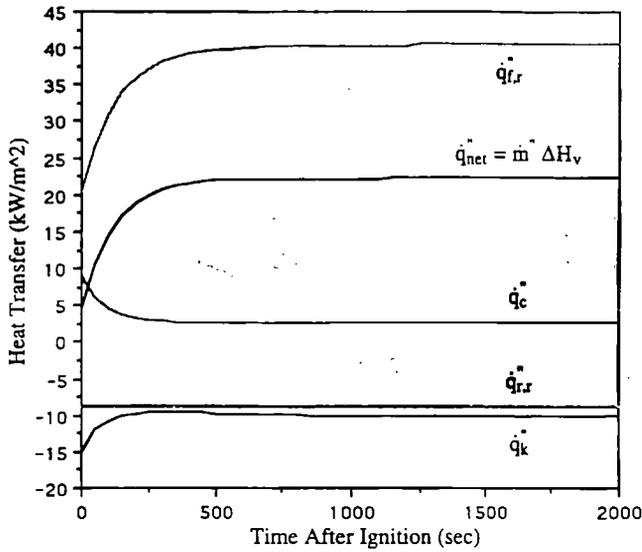
Figure 9. Heat transfer components for a turbulent pool fire 1.50 m<sup>2</sup> PMMA.
