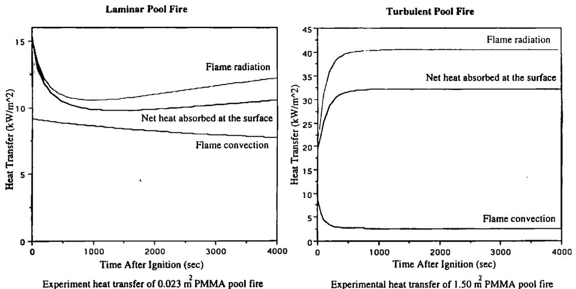
Figure 8. Comparison of experimental flame heat transfer results of 0.023 m<sup>2</sup> and 1.50 m<sup>2</sup> PMMA pool fires.
