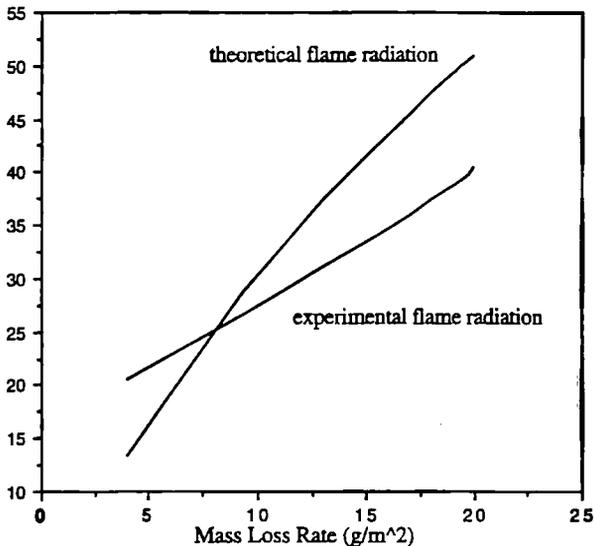
Figure 10. Experimental and theoretical flame radiative heat flux vs. mass loss rate of turbulent pool fire, 1.50 m<sup>2</sup> PMMA.
