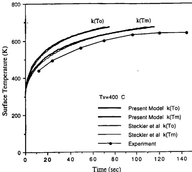
Figure 1. Surface temperature of PMMA exposed to 40 kW/m<sup>2</sup> incident heat flux.
