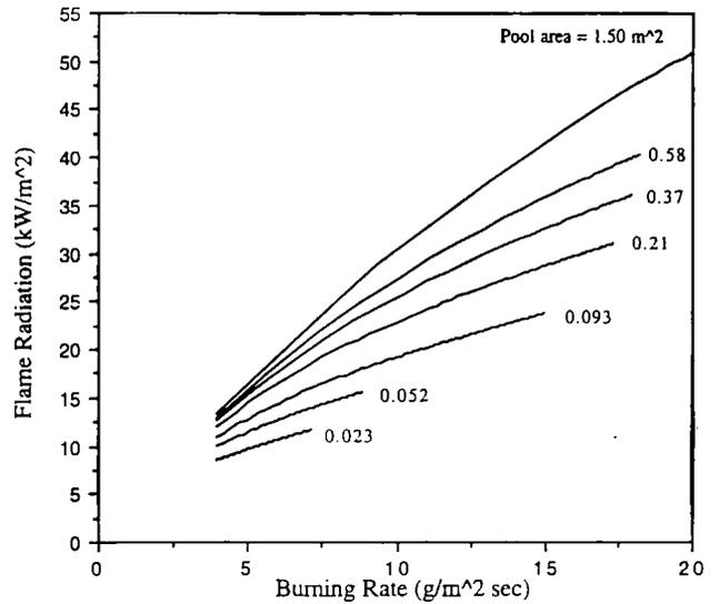
Figure 7. Experimental burning rate for seven square PMMA pool fires vs. Orloff and De Ris<sup>9</sup> flame radiation model.
