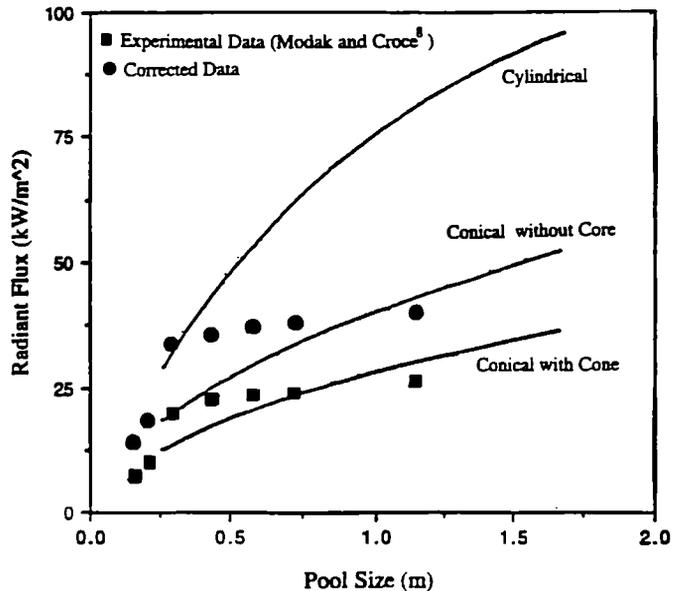
Figure 12. Corrected results of steady flame radiation to pool surface.
