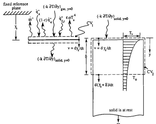
Figure 3. Model for a thermoplastic-like solid material.
