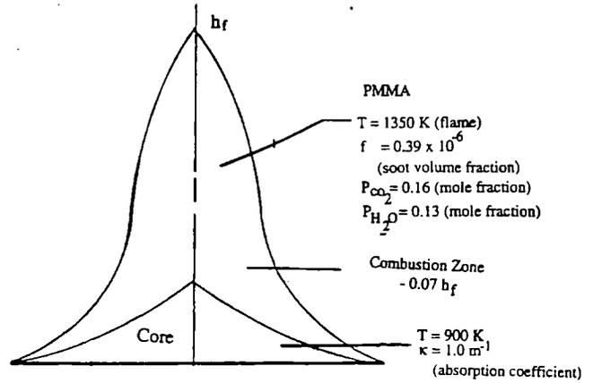
Figure 11. Radiative energy blockage in large pool fires, from Brosmer and Tien<sup>10</sup>.
