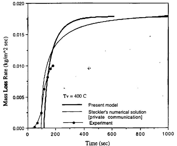
Figure 2. Mass loss rate of PMMA exposed to 40 kW/m<sup>2</sup> incident heat flux.
