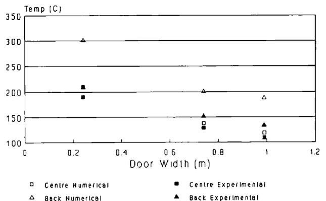
Figure 3b. Calculated and measured hot layer temperature (°C) as a function of door width (m) for centre and back positioned 62.9 kW fires.
