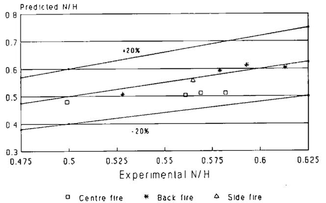
Figure 2b. Calculated and measured neutral plane height/door height for centre, back and side positioned fires. Model predictions use adiabatic boundary conditions.
