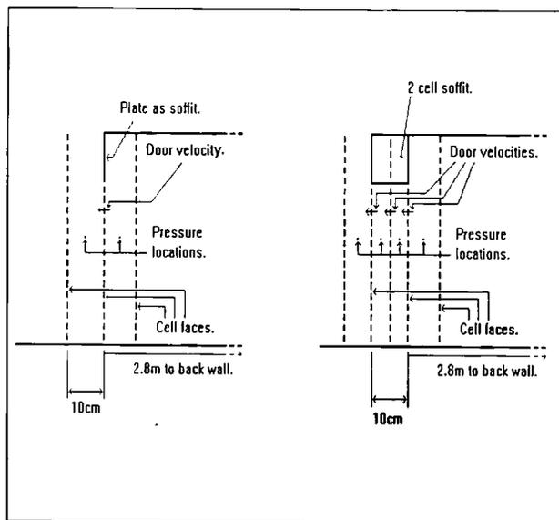
Figure 8. Velocity and pressure locations within doorway for PHOENICS models describing soffit as a zero thickness plate and a two cell thick soffit.
