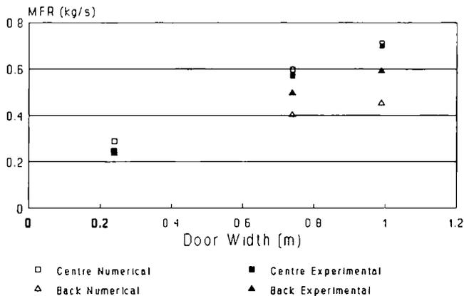
Figure 3d. Calculated and measured mass flux out (kg/s) as a function of door width (m) for centre and back positioned 62.9 kW fires.
