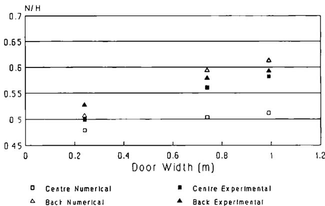
Figure 3a. Calculated and measured neutral plane height/door height as a function of door width (m) for centre and back positioned 62.9 kW fires.
