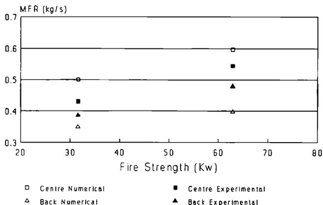
Figure 4c. Calculated and measured mass flux in (kg/s) as a function of fire size (kW) for centre and back positioned fires with 0.74 m wide door.
