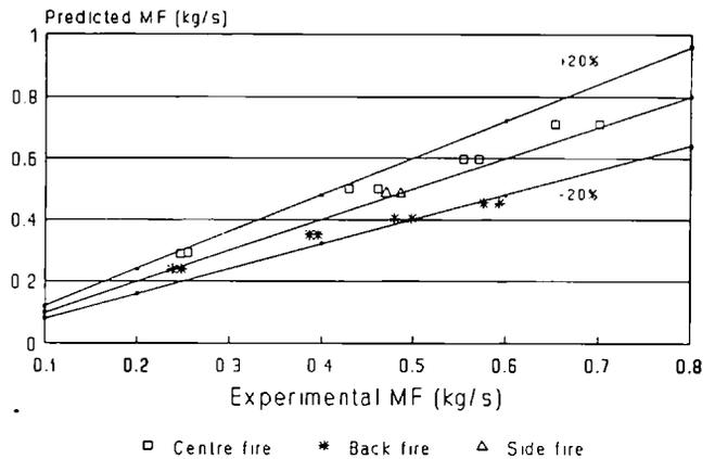
Figure 2c. Calculated and measured mass flux in and out (kg/s) for centre, back and side positioned fires. Model predictions use adiabatic boundary conditions.
