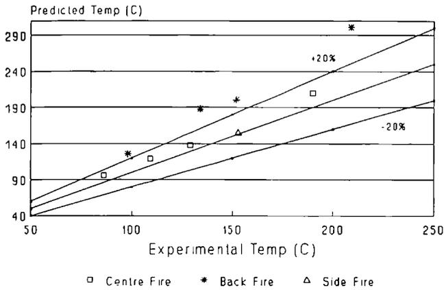
Figure 2a. Calculated and measured upper layer temperature ( $^{\circ}\text{C}$ ) for centre, back and side positioned fires. Model predictions use adiabatic boundary conditions.
