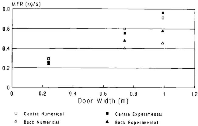
Figure 3c. Calculated and measured mass flux in (kg/s) as a function of door width (m) for centre and back positioned 62.9 kW fires.
