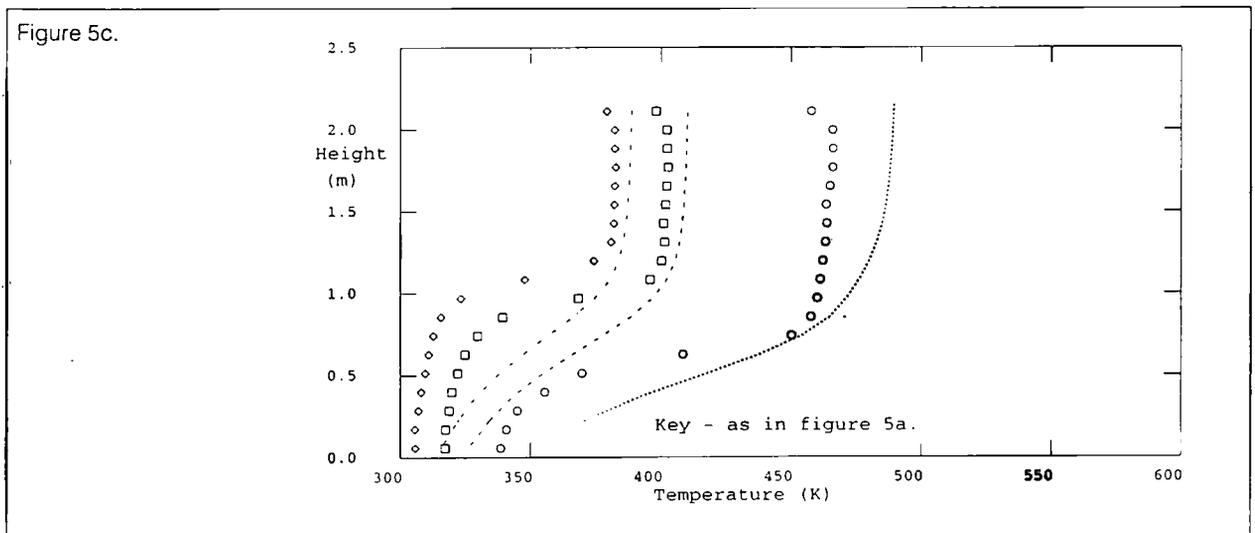
Figure 6. Predicted and measured (a) door centre vertical velocity profiles, (b) door centre vertical temperature profiles and (c) corner stack vertical temperature profiles for the 0.24m, 0.74m and 0.99m wide doors. In all cases, the 62.9 kW fire positioned adjacent to the rear wall was modelled.
