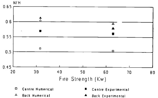
Figure 4a. Calculated and measured neutral plane height/door height as a function of fire size (kW) for centre and back positioned fires with 0.74 m wide door.
