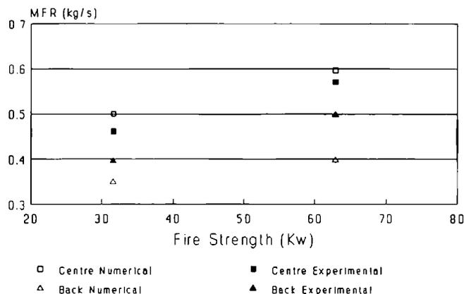
Figure 4d. Calculated and measured mass flux out (kg/s) as a function of fire size (kW) for centre and back positioned fires with 0.74 m wide door.
