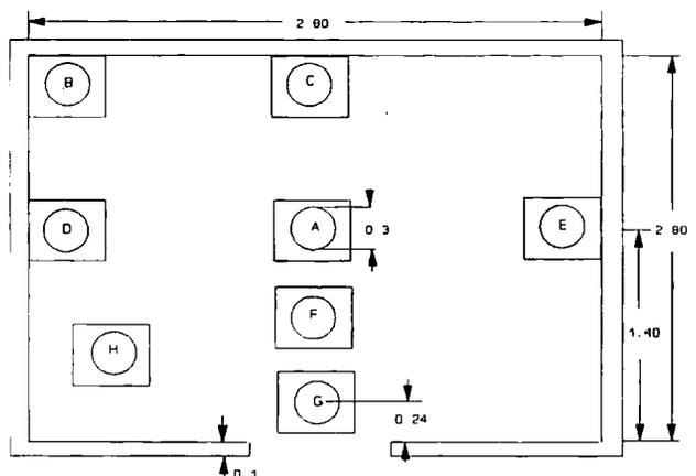
Figure 1. The eight fire locations studied in the experiments. Fires in locations A, C and D were simulated.
