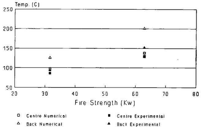
Figure 4b. Calculated and measured upper layer temperature (°C) as a function of fire size (kW) for centre, and back positioned fires with 0.74 m wide door.
