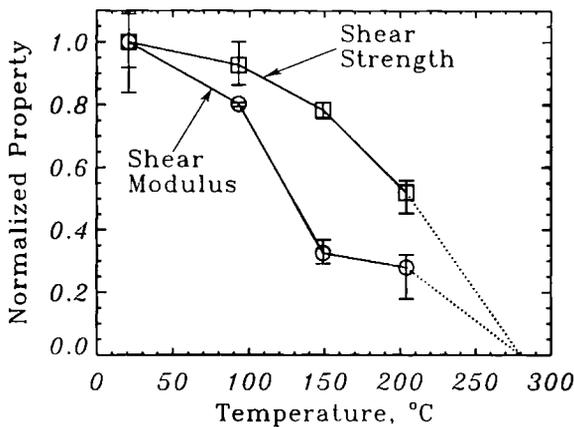
Figure 3 - Shear properties vs. temperature,
