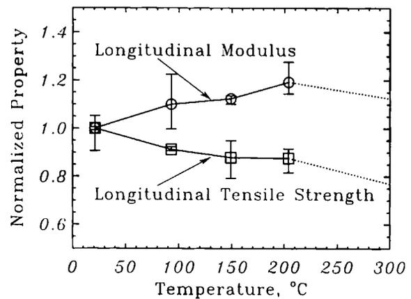
Figure 1 - Longitudinal properties vs. temperature.
