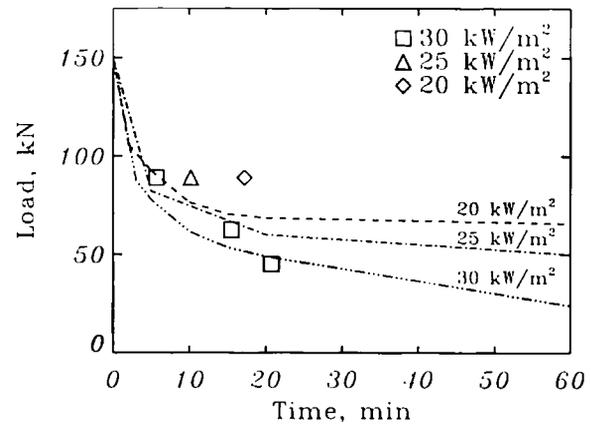
Figure 12 - Measured vs. predicted load vs. time-to-failure for  $[0/\neq 60/0)_{11}]_s$ .
