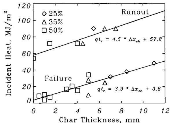
Figure 11 - Char thickness vs. thermal insult.
