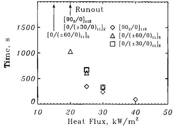
Figure 9 - Time-to-failure for 46% or 50% of ultimate load.
