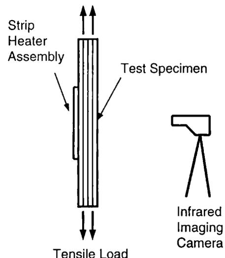
Figure 6 - Schematic diagram of experimental set-up for residual strength evaluation.
