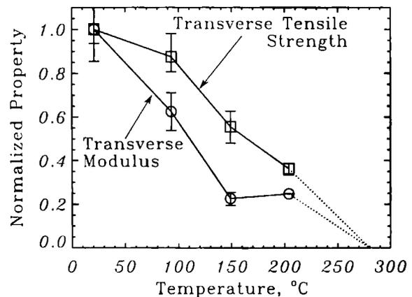
Figure 2 - Transverse properties vs. temperature.
