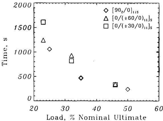
Figure 8 - Time-to-failure for 30 kW/m<sup>2</sup> heat flux.
