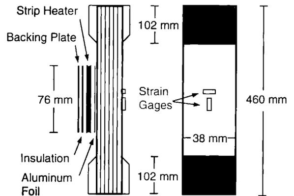
Figure 5 - Schematic diagram of residual strength specimen.
