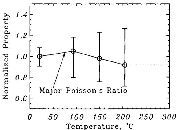
Figure 4 - Major Poisson's ratio vs. temperature.
