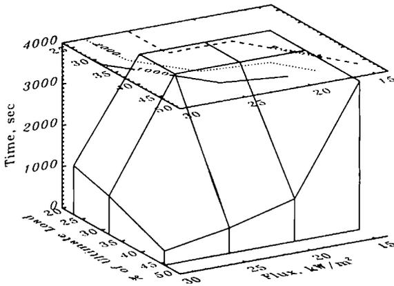
Figure 7 - Failure surface of  $[0/(\pm 60/0)_{11}]_s$ .
