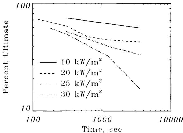
Figure 13 - Predicted load vs. time-to-failure for  $[0/(\neq 60/0)_{11}]_s$ .
