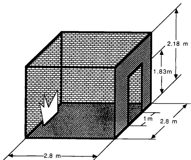
Figure 1: Three dimensional view of the fire compartment.
