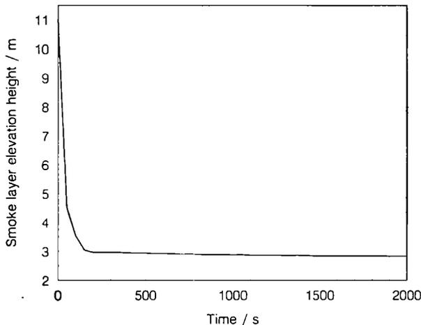
Figure 3. Smoke layer elevation height at the atrium.
