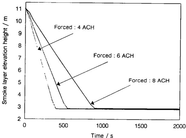
Figure 8. Effect of forced ventilation on the smoke layer elevation height at the atrium without upper levels.
