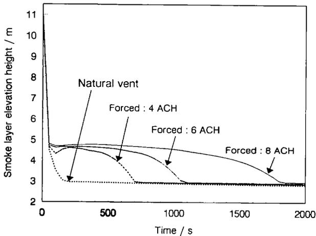
Figure 7. Effect of ventilation on the smoke layer elevation height at the atrium.
