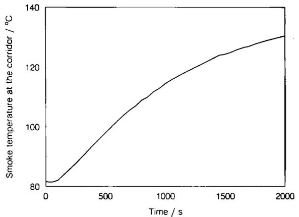
Figure 5. Smoke temperature at the upper corridor for shops (rooms 3 and 4).
