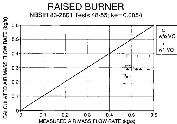
Figure 3d. Calculated and measured air mass flow rates for raised fires.  $k_e = 0.0054$ . (w/VO means with virtual origin; w/o VO means without virtual origin).
