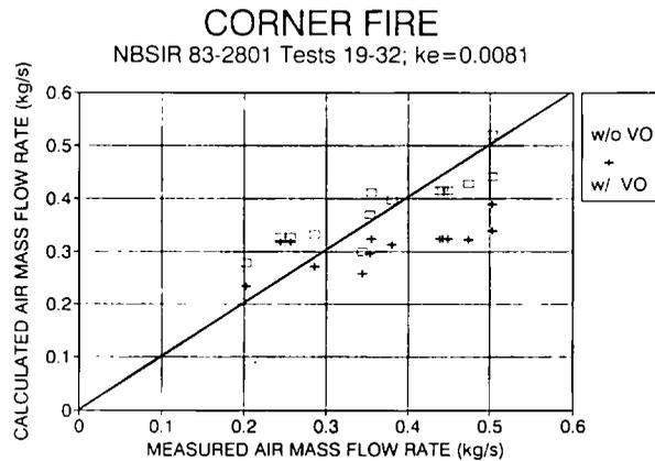
Figure 4b. Calculated and measured air mass flow rates for corner fires.  $k_e = 0.0081$ . (w/VO means with virtual origin; w/o VO means without virtual origin).
