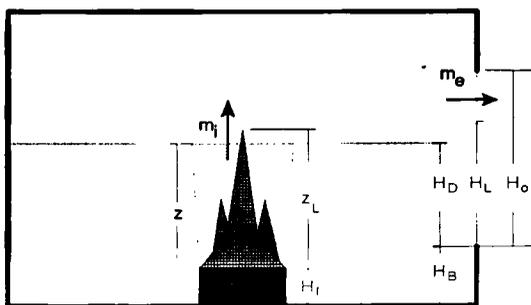
Figure 1. The naturally ventilated room fire geometry.
