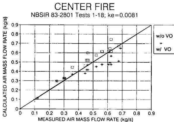
Figure 4a. Calculated and measured air mass flow rates for center fires.  $k_e = 0.0081$ . (w/VO means with virtual origin; w/o VO means without virtual origin).
