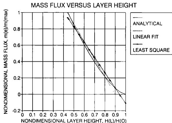
Figure 2. Comparison of exact and approximate mass flux rates as a function of the nondimensional layer height.
