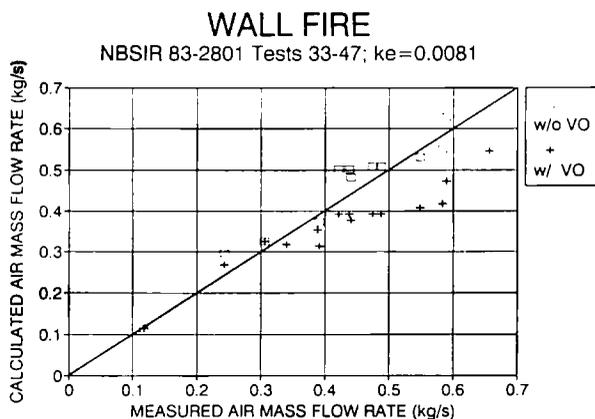
Figure 4c. Calculated and measured air mass flow rates for wall fires.  $k_e = 0.0081$ . (w/VO means with virtual origin; w/o VO means without virtual origin).
