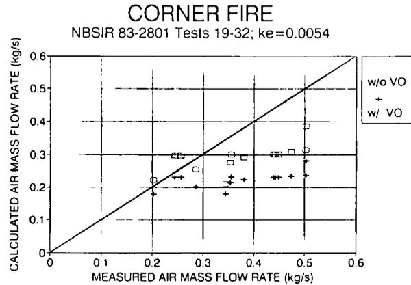
Figure 3b. Calculated and measured air mass flow rates for corner fires.  $k_e = 0.0054$ . (w/VO means with virtual origin; w/o VO means without virtual origin).
