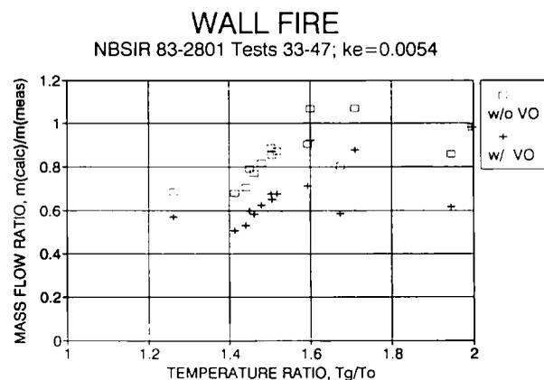
Figure 5b. Mass flow ratio as a function of the temperature ratio for wall fires.  $k_e = 0.0054$ . (w/VO means with virtual origin; w/o VO means without virtual origin).
