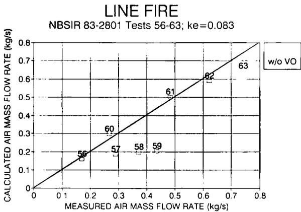
Figure 3e. Calculated and measured air mass flow rates for line fires.  $k_e = 0.083$ . (w/o VO means without virtual origin).
