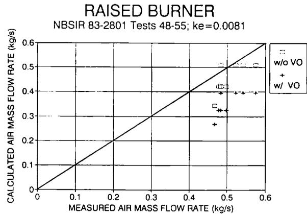
Figure 4d. Calculated and measured air mass flow rates for raised fires.  $k_e = 0.0081$ . (w/VO means with virtual origin; w/o VO means without virtual origin).
