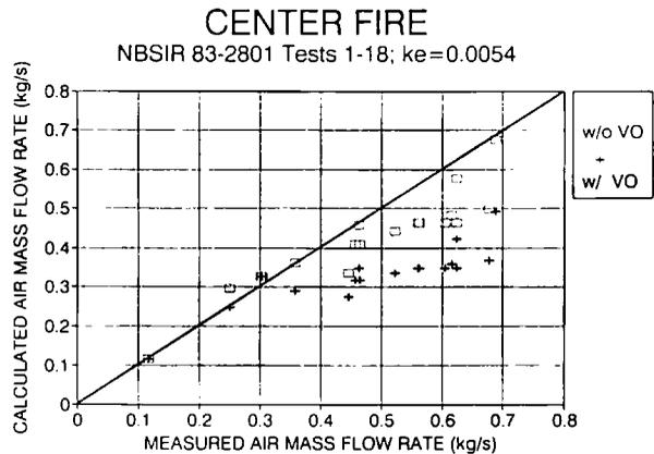
Figure 3a. Calculated and measured air mass flow rates for center fires.  $k_e = 0.0054$ . (w/VO means with virtual origin; w/o VO means without virtual origin).
