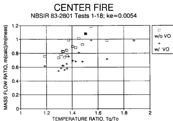
Figure 5a. Mass flow ratio as a function of the temperature ratio for center fires.  $k_e = 0.0054$ . (w/VO means with virtual origin; w/o VO means without virtual origin).
