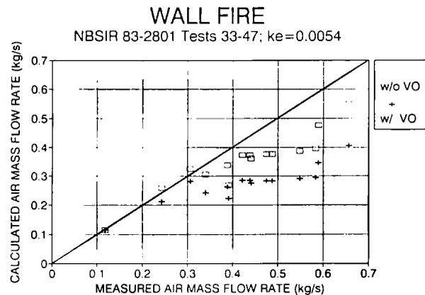
Figure 3c. Calculated and measured air mass flow rates for wall fires.  $k_e = 0.0054$ . (w/VO means with virtual origin; w/o VO means without virtual origin).
