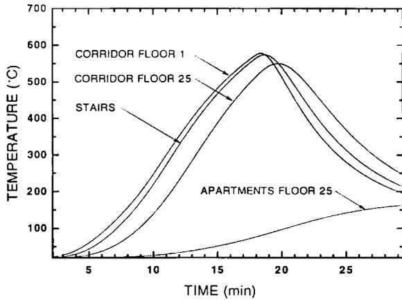
Figure 8. Temperature development at various locations in the building for a non-flashover fire with door open on first floor.
