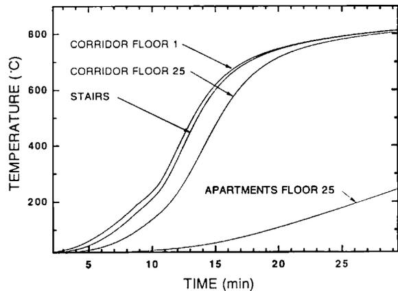
Figure 4. Temperature development at various locations in the building for a fully developed fire with door open on the first floor.
