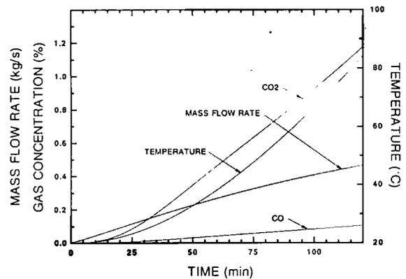
Figure 11. Conditions in apartment of fire for a smouldering fire.
