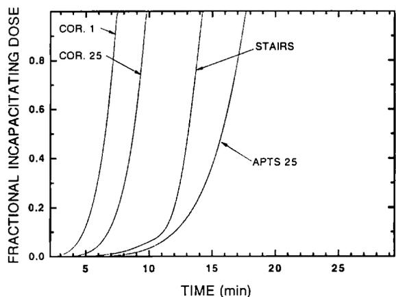
Figure 5. FID values at various locations in the building for the fully developed fire with door open on the first floor.
