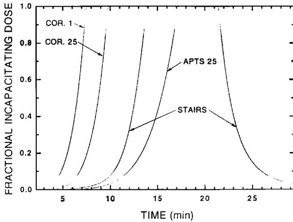
Figure 9. FID values at various locations in the building for a non-flashover fire with door open on the first floor.
