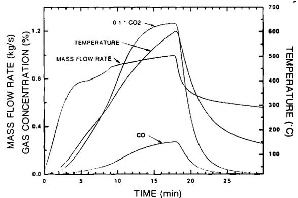
Figure 7. Conditions in apartment of fire for a non-flashover fire with door open.
