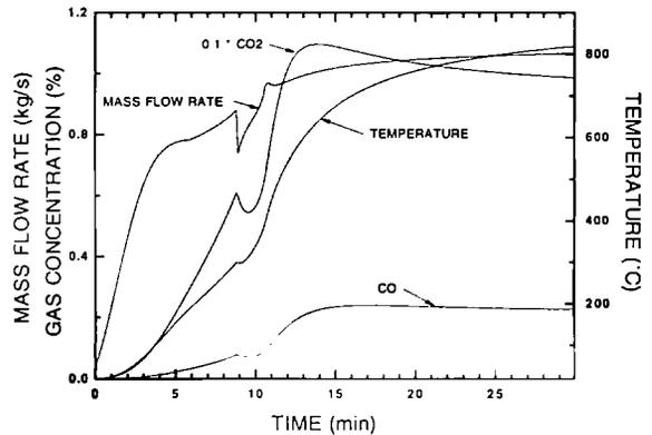
Figure 3. Conditions in apartment of fire for a fully developed fire with door open.
