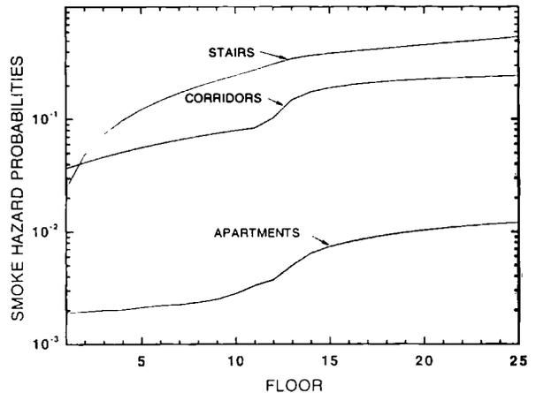
Figure 6. Smoke hazard probabilities on each floor in the building due to fully developed fires on each floor.
