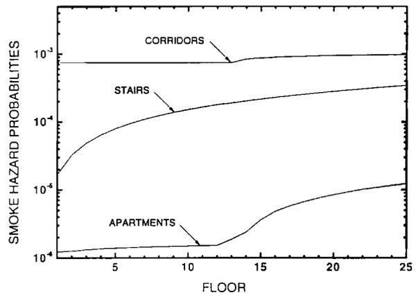
Figure 12. Smoke hazard probabilities at each floor in the building due to smouldering fires on each floor.
