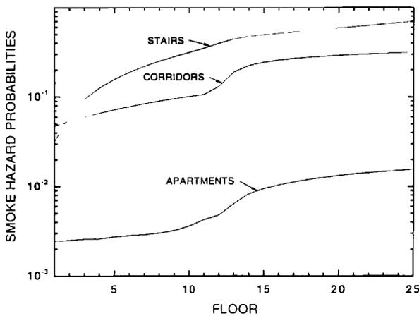
Figure 10. Smoke hazard probabilities at each floor in the building due to non-flashover fires on each floor.
