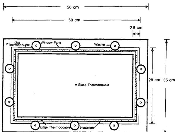
Figure 2. Schematic of window installation including thermocouple placement.
