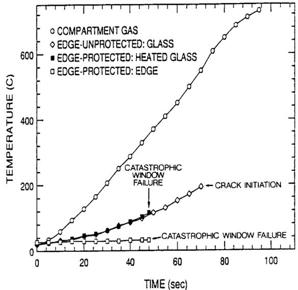
Figure 3. Time-temperature history of glass for 20 cm x 30 cm pan fire for both edge-protected (Test 3) and edge-unprotected (Test 14) installations.
