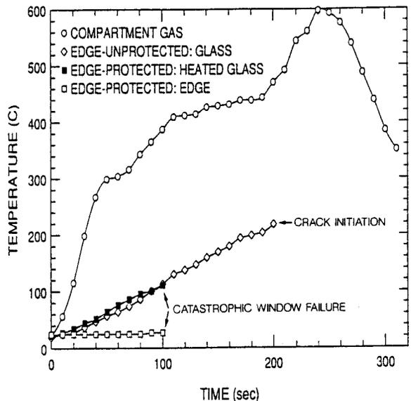
Figure 4. Time-temperature history of glass for 20 cm x 20 cm pan fire for both edge-protected (Test 4) and edge-unprotected (Test 15) installations.
