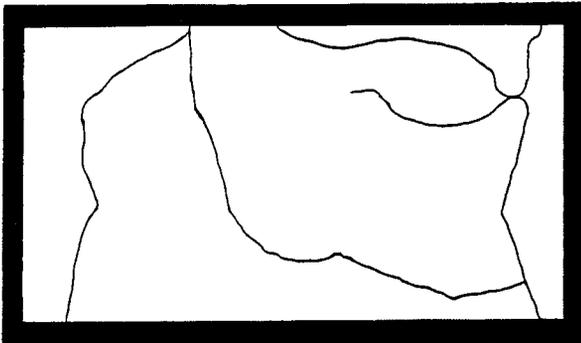
Figure 6. Diagram of the window breakage pattern for two edge-protected tests (top: Test 2; Bottom: Test 7).
