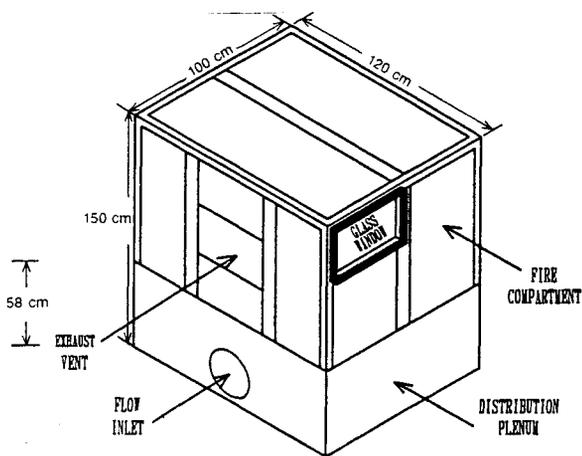
Figure 1. Schematic of the compartment used for window breakage tests.
