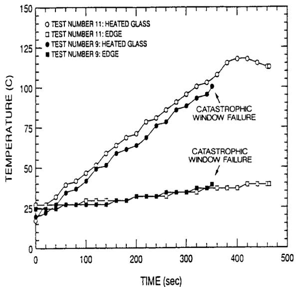
Figure 5. Time-temperature history of glass for 10 cm x 20 cm pan fire for two edge-protected installations (Test 9, with glass breakage and Test 11, with no glass breakage).
