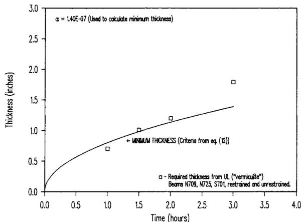
Figure 2. Required insulation thickness.
