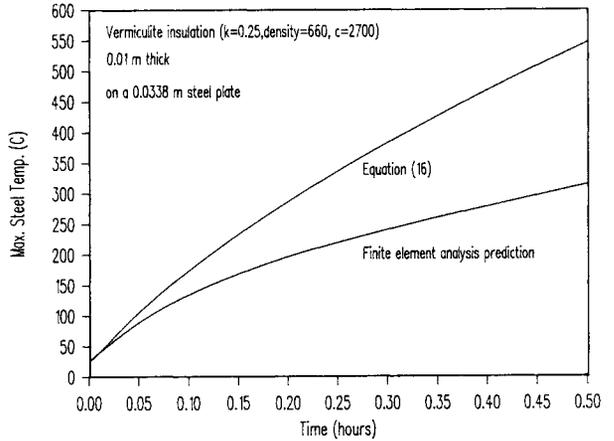
Figure 3. Steel temperature prediction; 0.01 m insulation.
