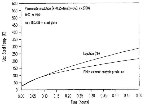
Figure 4. Steel temperature prediction; 0.02 m insulation.
