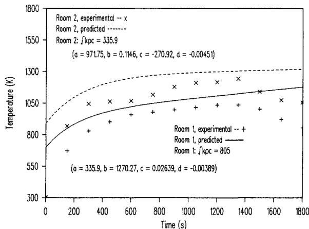
Figure 1. Predicted vs. experimental fire temperature.
