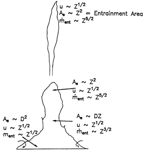
Figure 4: A turbulent jet flame and a pool fire configuration for which the present results for the buoyant plume above the flame tip are applicable ( $Z_f \gtrsim D/2$ ).
