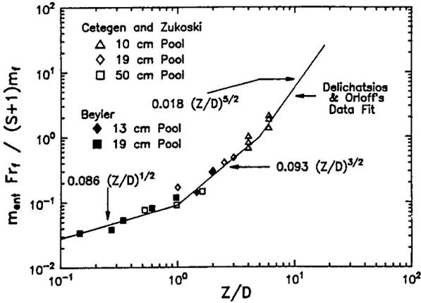
Figure 1: Air entrainment rates into turbulent jets and pool fires below the flame tip.
