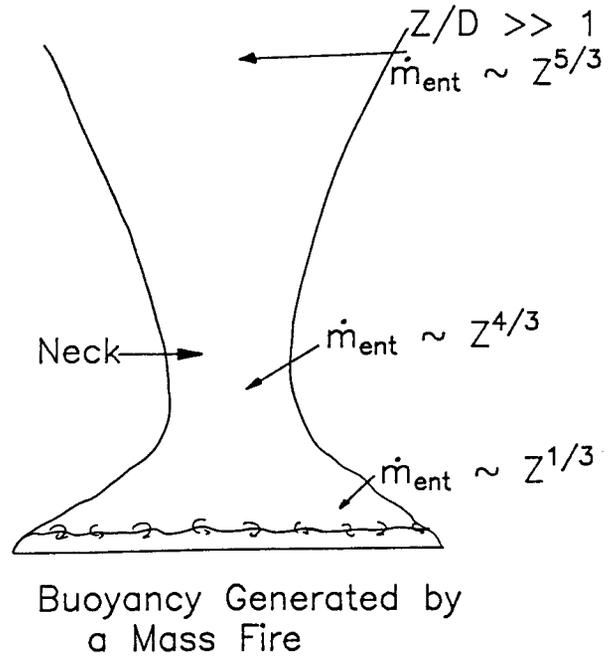
Figure 5: A very large pool fire ("mass" fire) situation for which the present results for the buoyant plume above the flame tip are not applicable ( $Z_f < D/2$ ). In a "mass" fire situation the flame height is independent of the pool diameter and depends only on the heat release rate per unit area (this situation is included in the first flame height equation of Section II.1.a.2).
