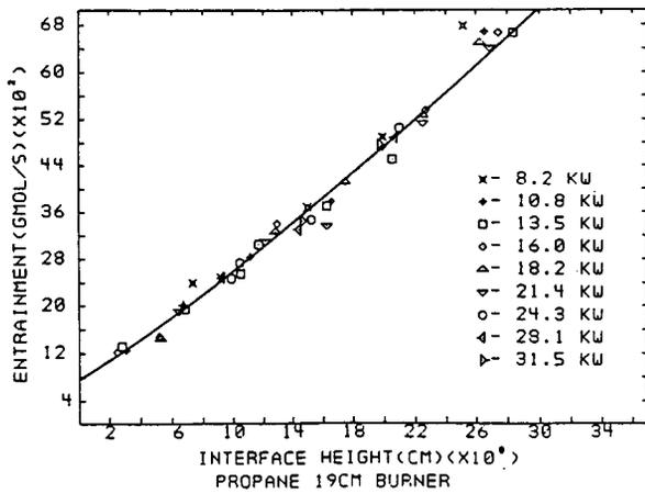
Figure 2: Air entrainment into a 19 cm propane burner pool fire below the flame tip. These results illustrate that air entrainment is independent of heat release rate,  $Q$  (taken from Reference 2).
