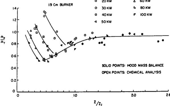
Figure 3: Air entrainment into the buoyant plume above the flame tip (taken from Reference 3). The reference value,  $\dot{m}_7$ , in the ordinate is given by Equation 1 in the text.
