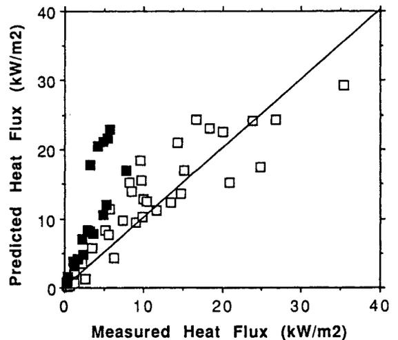
Figure 5. Comparison of the radiant heat flux predicted by the Mudan & Croce method with the experimental data from References 1-4, 6. Solid symbols are data points which are overpredicted by more than a factor of two.
