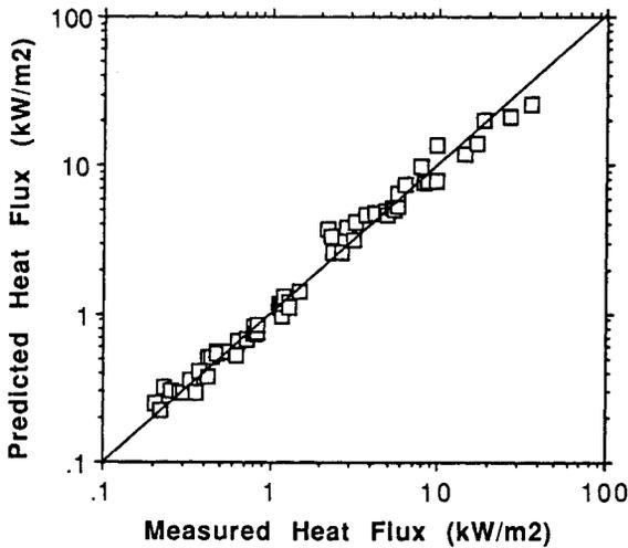
Figure 1. Comparison of calculated and measured incident radiant flux using the 'effective' emissive powers from Table 1. The solid line indicates equality of the predicted and measured heat fluxes.
