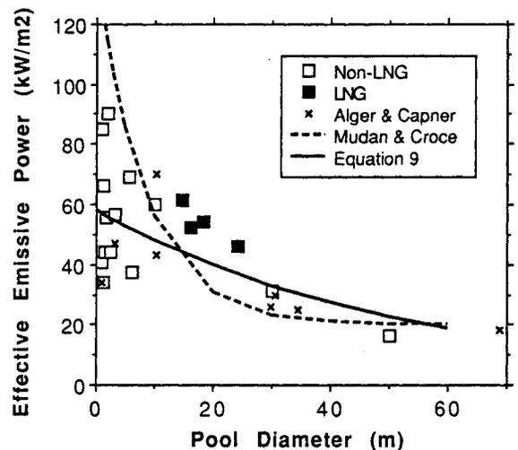
Figure 3. 'Effective' emissive power as a function of the pool diameter. Solid symbols are LNG experiments. The solid line is Equation 9, a curve fit to the present results, and the dashed line is Equation 10<sup>23</sup>. The '+'s are results derived from Alger and Capner<sup>27</sup>.
