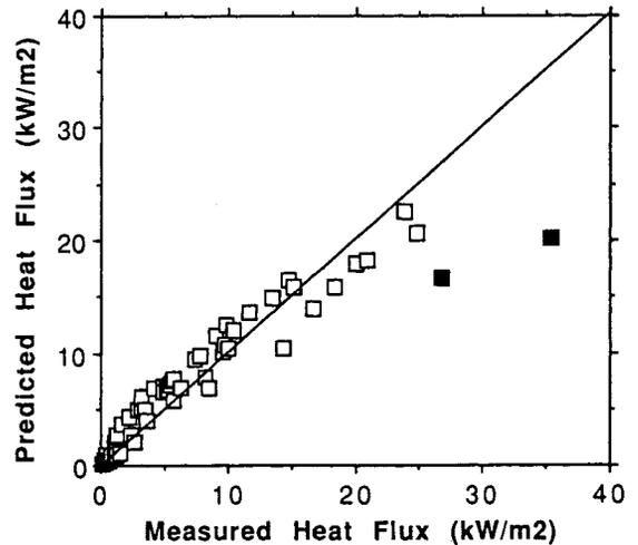
Figure 4. Comparison of the radiant heat flux predicted by the present method with the experimental data from References 1-4, 6. Solid symbols are data points which are underpredicted by more than 35%.
