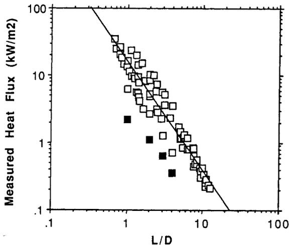
Figure 2. Measured incident radiant flux at ground level to a vertical target as a function of the distance from the pool center to the target normalized by the pool diameter. Solid symbols are 50 m diameter kerosene data. The solid line is Equation 8.
