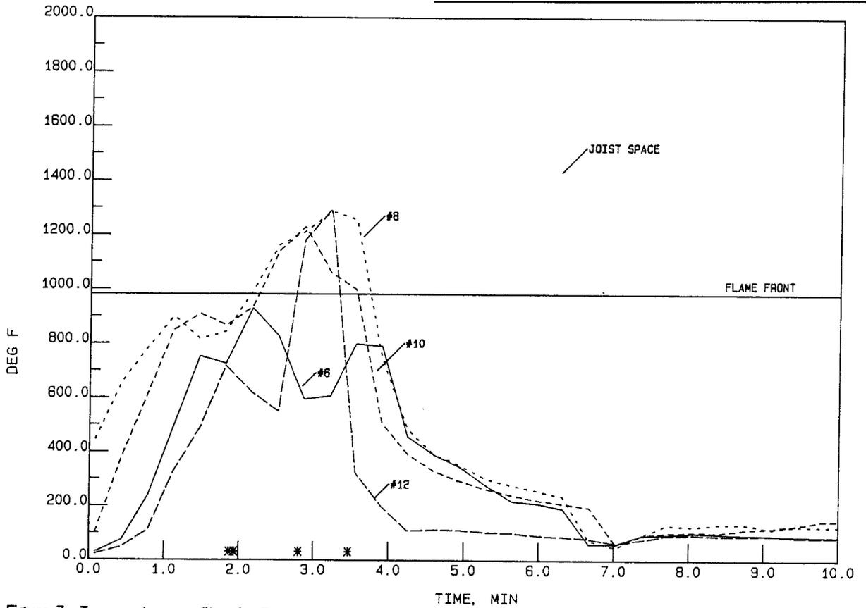
Figure 7. Temperature profiles for Test 1 measured 21 ft (6.4 m) from the south end.
