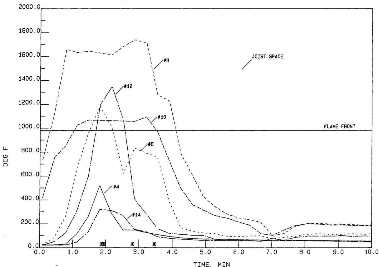
Figure 4. Temperature profiles for Test 1 measured 3 ft (0.9 m) from the south end.
