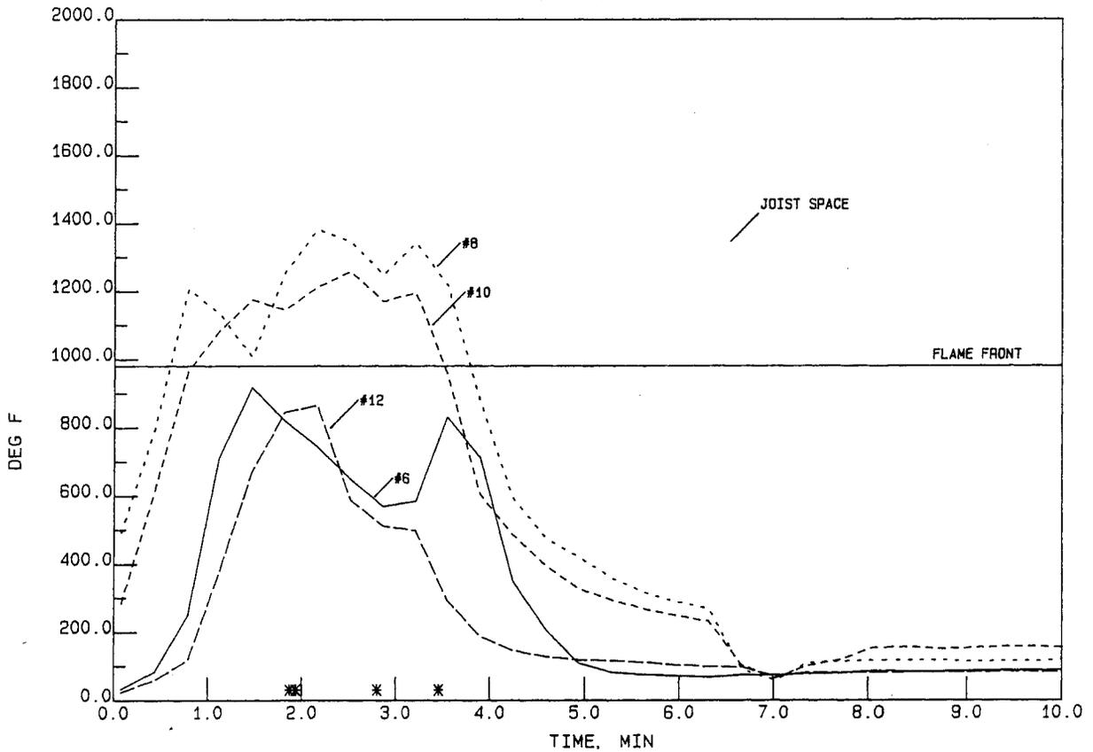
Figure 6. Temperature profiles for Test 1 measured 15 ft (4.6 m) from the south end.
