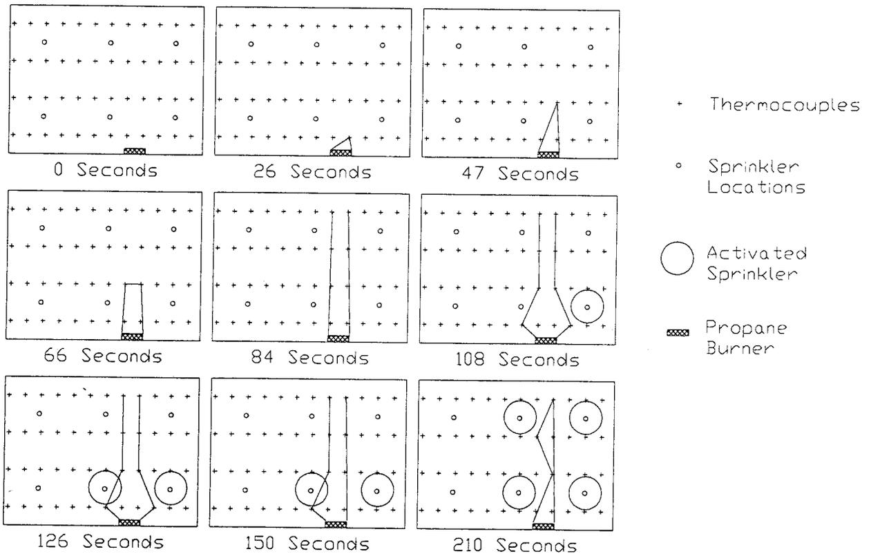
Figure 8. Flame extent at various times for Test 1.
