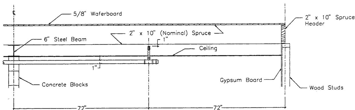
Figure 2. Cross-section of the ceiling assembly viewing normal to the joists showing the relative position of the sprinkler.
