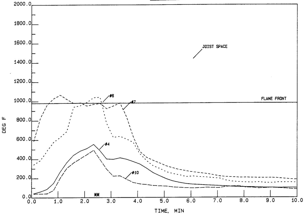
Figure 13. Temperature profiles for Test 2 measured 21 ft (6.4 m) from the south end.
