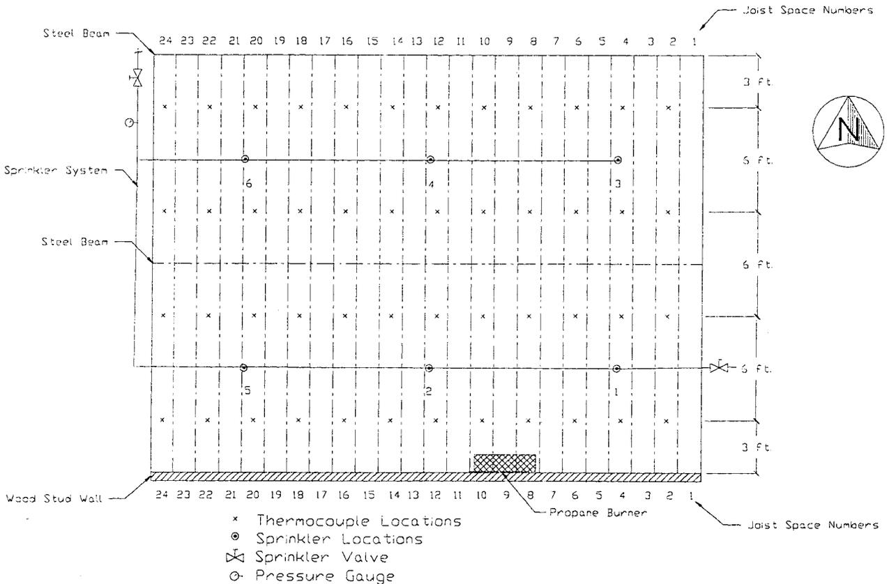
Figure 1. Plan view of the ceiling assembly showing the location of the propane burner, sprinklers and thermocouples for Test 1.
