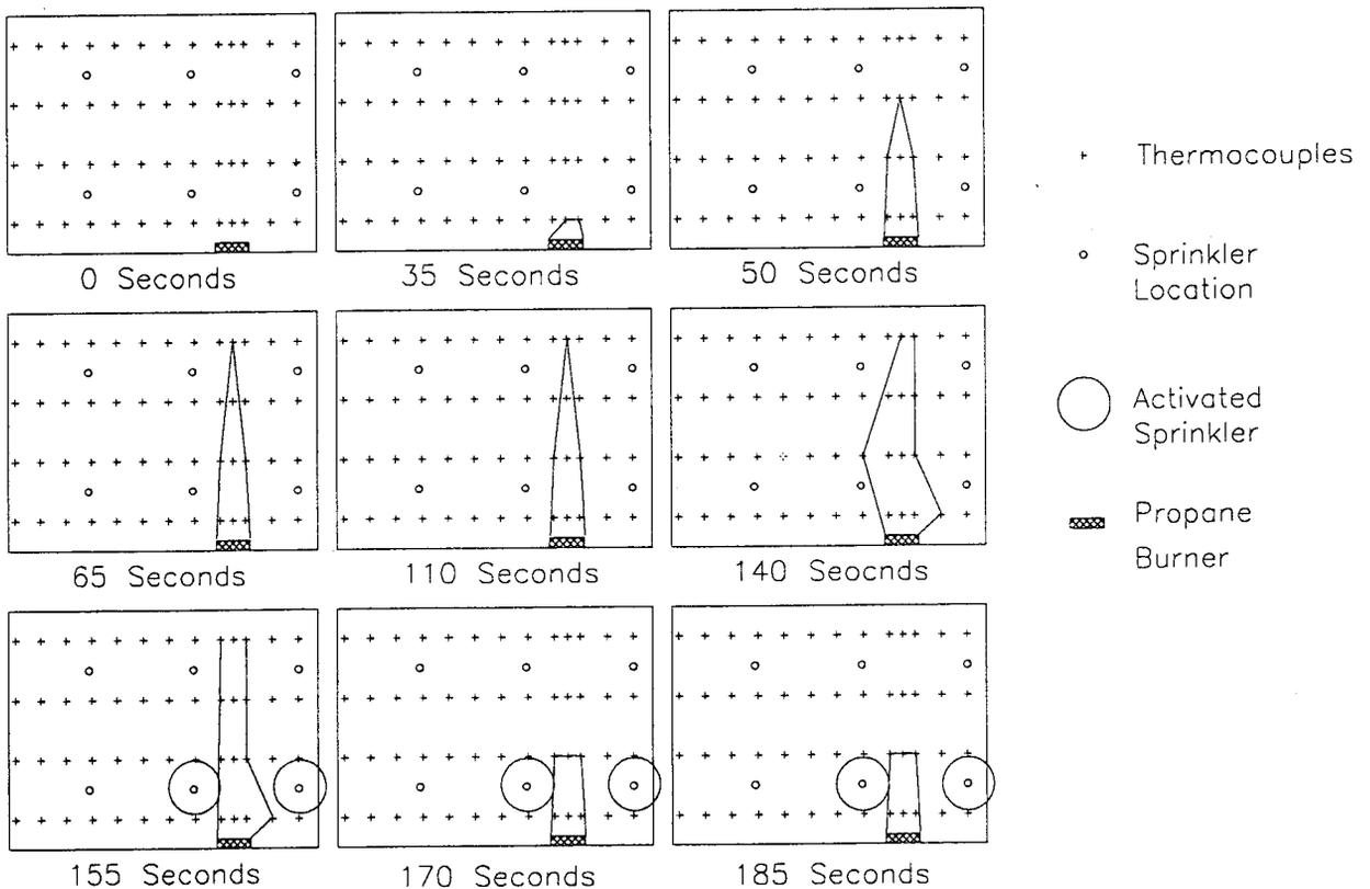
Figure 14. Flame extent at various times for Test 2.
