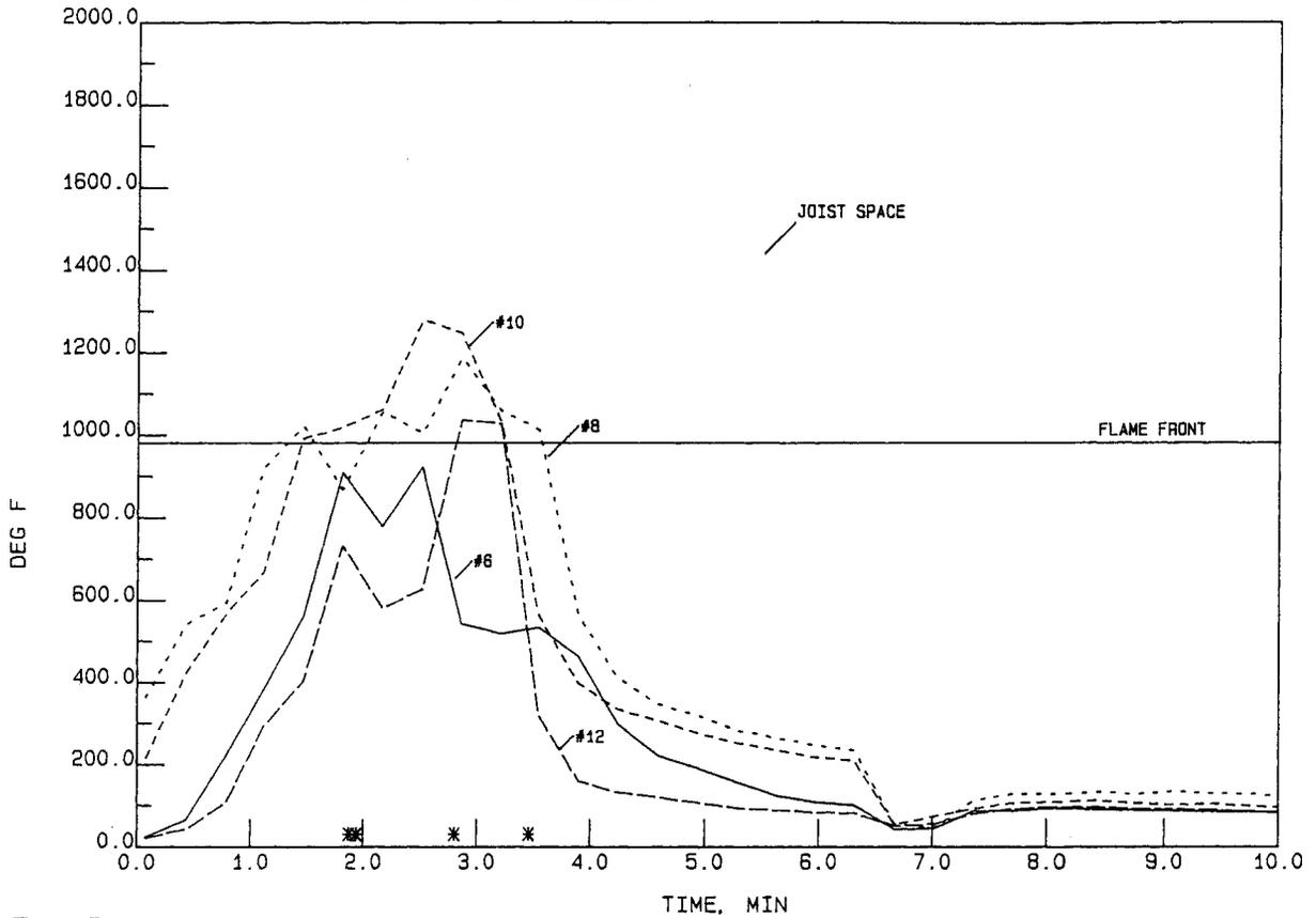
Figure 5. Temperature profiles for Test 1 measured 9 ft (2.7 m) from the south end.
