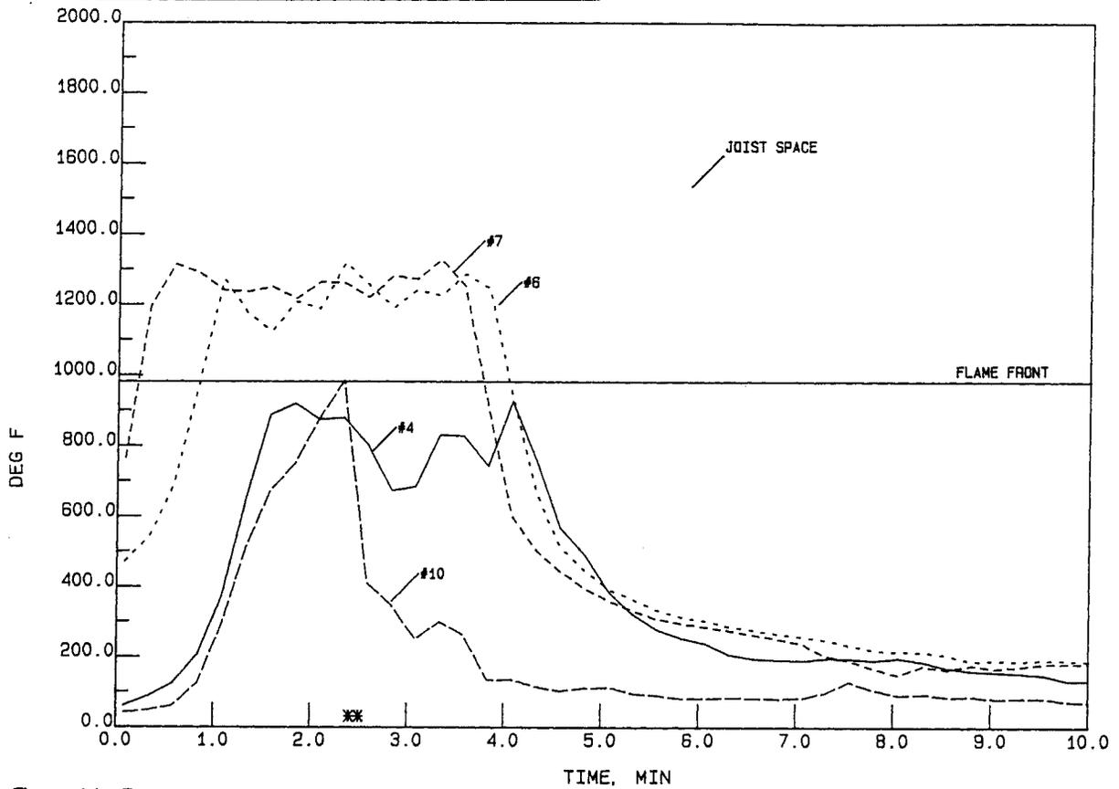
Figure 11. Temperature profiles for Test 2 measured 9 ft (2.6 m) from the south end.
