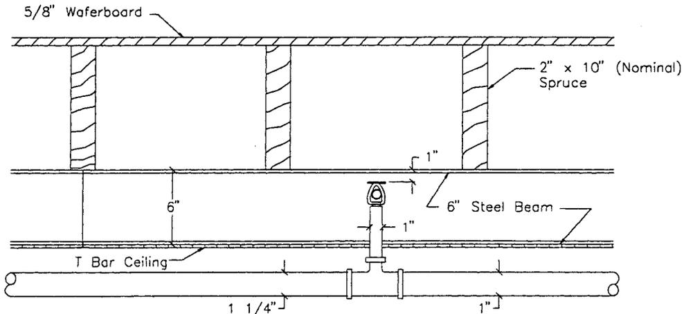
Figure 3. Cross-section of the ceiling assembly viewing parallel to the joists showing the relative positions of the sprinklers.
