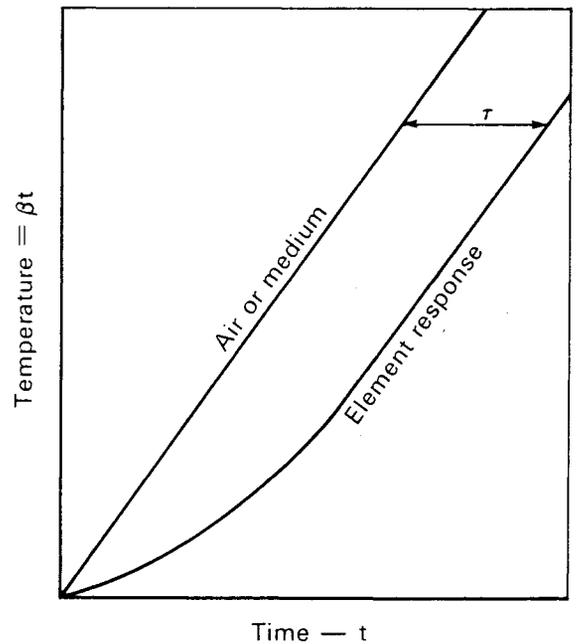
(b) Ramp (linear rate of rise)  $\beta t$  °C/min
