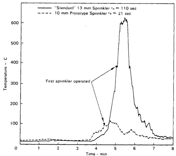
Figure 12. Comparison of gas temperature at first sprinkler location in living room.
