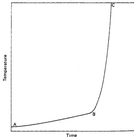
Figure 2. Fire growth in life safety and high rack situations (schematic).
