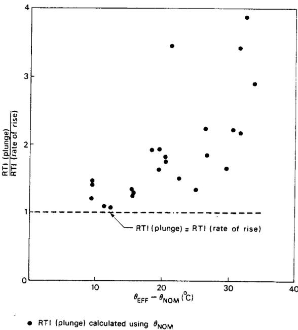
Figure 6. Summary of experimental results showing the ratio of the RTI values measured in the rate of rise and plunge tests.
