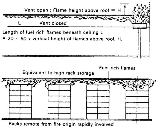
Figure 1. Horizontal length of flames below ceiling equivalent to vertical height of flames above roof for fires burning at high and low levels.
