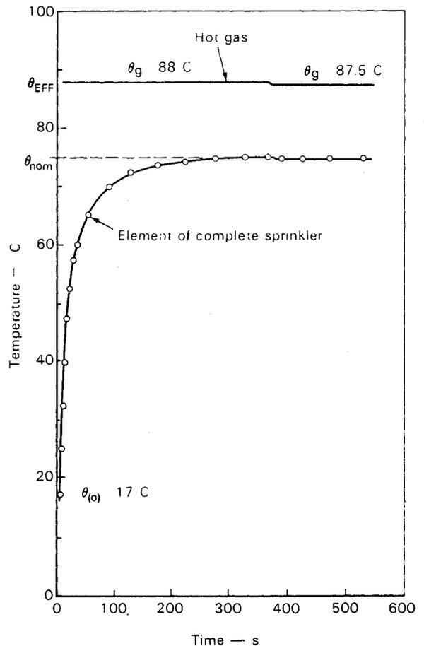
Figure 8. Link temperatures: plung test (wet) at  $q_E$ .
