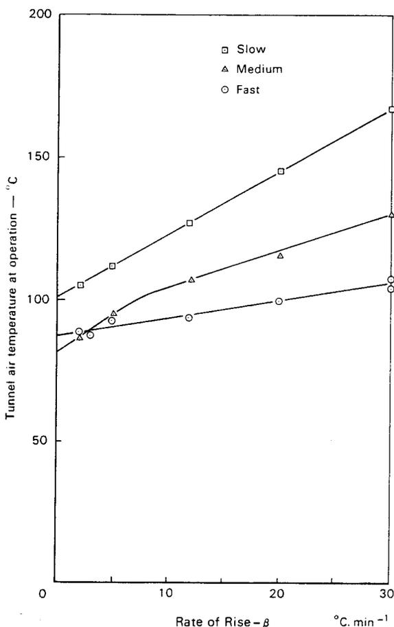
Figure 9. Rate of rise test results for slow, medium and fast response sprinklers.
