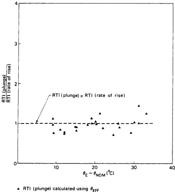
Figure 7. Summary of experimental results showing the ratio of the plunge and rate of rise  $RTI$  values based on effective operating temperature.
