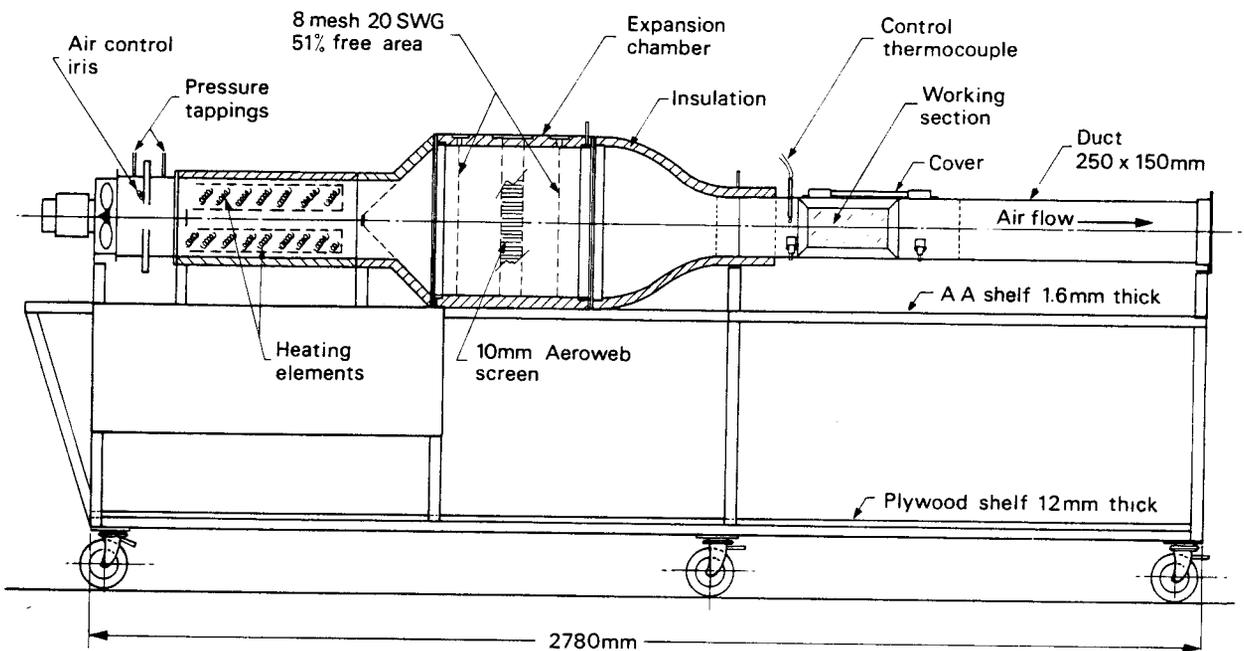
Figure 3. FRS heated wind tunnel.
