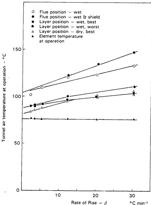
Figure 11. Rate of rise test results for fast response sprinkler.
