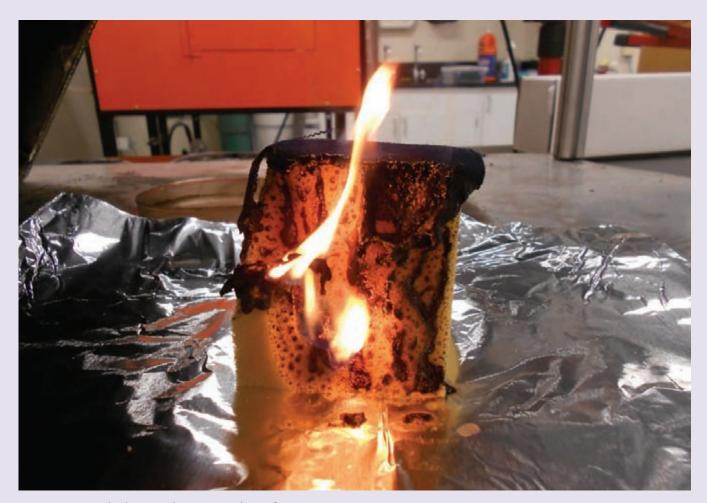
Figure 5: Foam and Fabric Sample Sustaining Flame After Ignition
