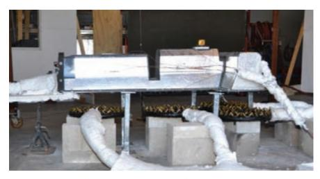
Figure 1: Battery B configuration and burner locations for HRR testing
