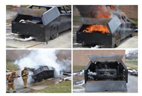
Figure 4: Test A3: Ignition of propane burners (top left); rear involved (top right); initial suppression activities (bottom left); suppression complete (bottom right)
