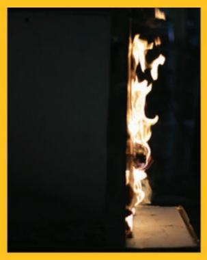
Figure 3: (left) Front video footage during a representative test. The blue contour across the width indicates the measured height of the pyrolysis region. (right) Image taken from the side of a sample during a representative test. Curling of the front layer of cardboard is visible in both images, but the extent of three-dimensional effects is more clearly seen in the side image.<sup>5</sup>
