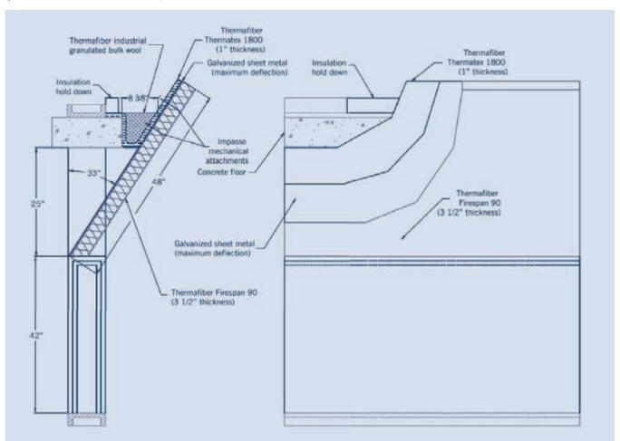
Figure 3. Drawing of the small-scale furnace test set-up (used with permission from Thermafiber Inc.)
