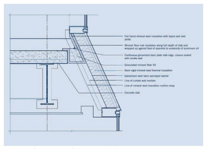
Figure 1. Perimeter fire containment concept for the twisting spandrel conditions
