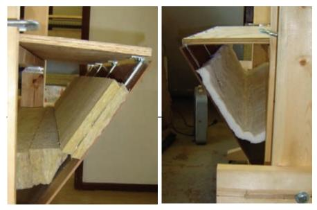
Figure 2. (Left) Detailed mock-up using mineral wool installed along the 30° inclined spandrel back pan. (Right) Detailed mock-up using needled mineral wool blanket also installed along the 30° inclined spandrel back pan. (Both figures are used with permission from Thermafiber Inc.)
