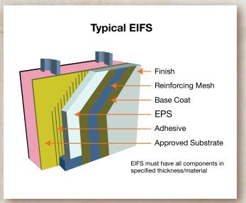
Figure 2. Components of an Exterior Insulation and Finish System (EIFS)
