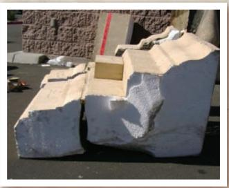
Figure 4. Sample taken from the horizontal band at the 29th floor
