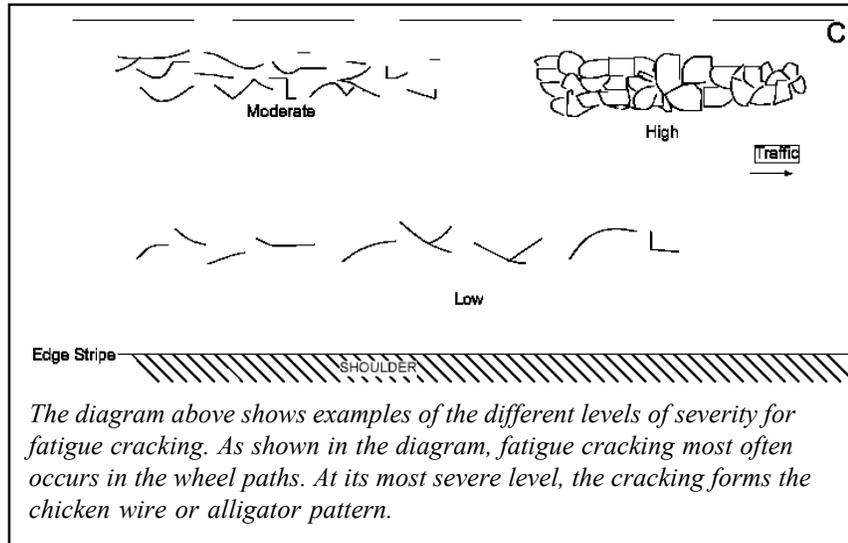
*The diagram above shows examples of the different levels of severity for fatigue cracking. As shown in the diagram, fatigue cracking most often occurs in the wheel paths. At its most severe level, the cracking forms the chicken wire or alligator pattern.*
