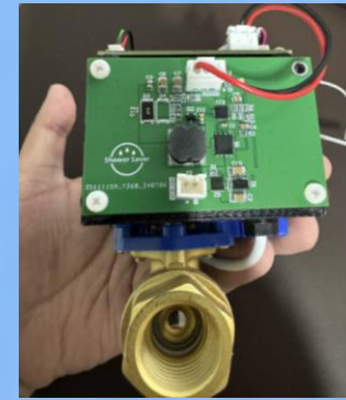
Interior View (PCBs & Battery Supply)
