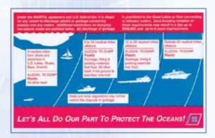
United States ocean-going vessels of 40 feet or longer that are engaged in commerce or equipped with a galley and berthing must have a written waste management plan describing the procedures for collecting, processing, storing, and discharging garbage, and must designate the person in charge of carrying out the plan.
