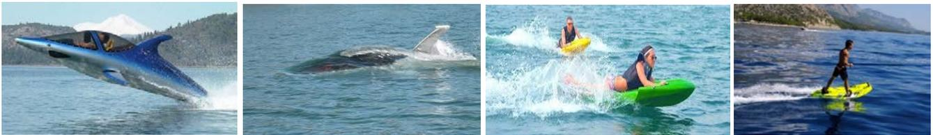
The Seabreacher operates at the surface, it can dive underwater for brief periods of time (10 seconds to 1 minute), and can also launch above the surface of the water like a breaching whale. It is a vessel, but wouldn’t likely be considered a PWC as the operator rides “in” the vessel.
