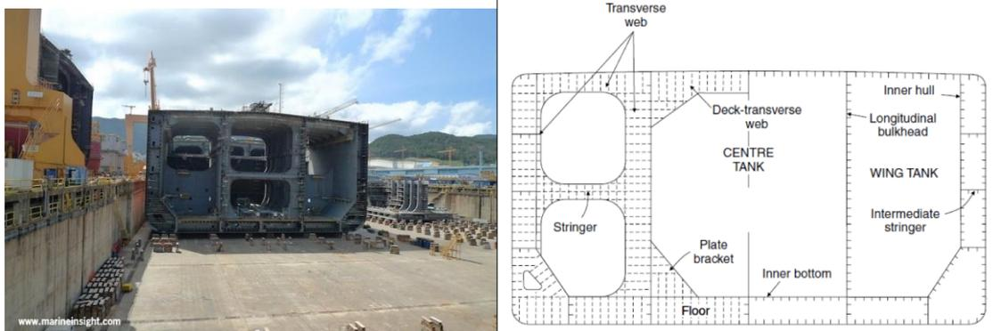
*Cross section of – Double Hull Oil Tanker*
