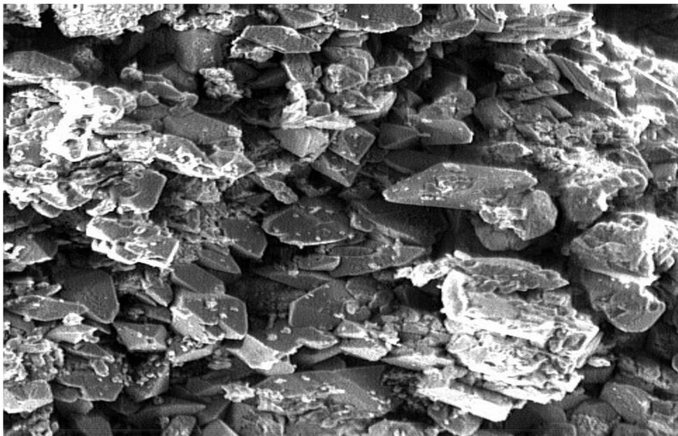
*Fully formed Sulphur Crystals as found on rust samples from cargo tanks*
