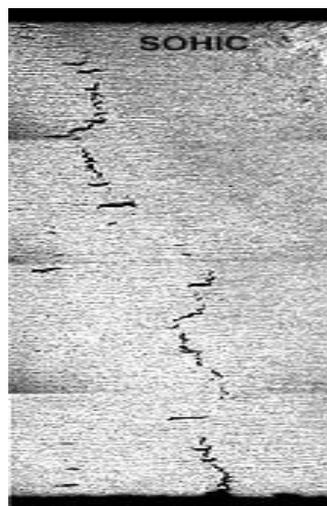
*The second type produces an array of blister cracks linked in the through thickness direction by trans-granular, cleavage cracks. The latter type of cracking is referred to as Stress Oriented Hydrogen Induced Cracking (SOHIC). SOHIC can have a greater effect of serviceability than HIC since it effectively reduces load carrying capabilities to a greater degree”<sup>1</sup>*
