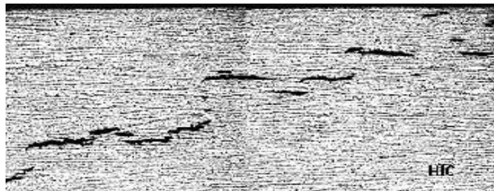
*Wet H<sub>2</sub>S cracking can occur in susceptible steels exposed to aqueous environments containing hydrogen sulphide. It is a form of hydrogen-related cracking and can have two distinct morphologies: The first type is commonly referred to as Hydrogen Induced Cracking (HIC) and can occur where little or no applied or residual tensile stress exists. It is manifested as blisters or blister cracks oriented parallel to the plate surface.*
