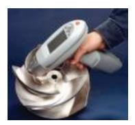
Photo of an XRF Alloy Analyzer (Niton)
