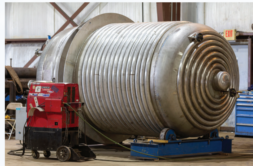
Apex Engineered Product provides multi-stage reactor fabrication consisting of Hastelloy C-276 vessel and internals and 316 SS water jacket.
