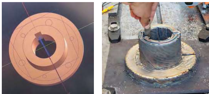
(Left) Computer-aided design of reverse osmosis shaft collet. Photo courtesy of Mr. Jacob Lopez, NSWC Corona. (Right) Part just after printing. Photo courtesy of LT Charles Wallace, NPS.
