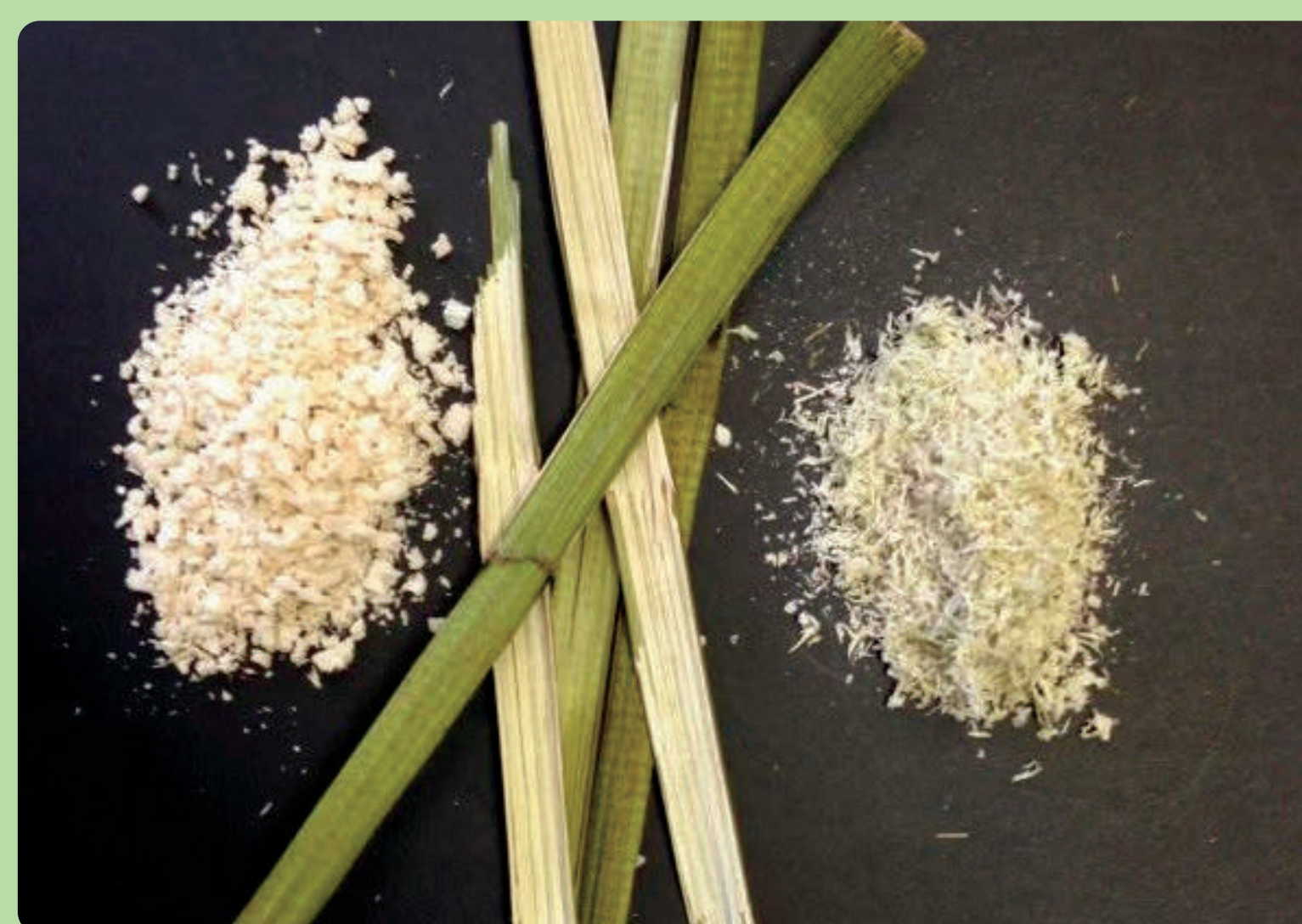
Kenaf decorticated into fibre & hurd (QLD)
