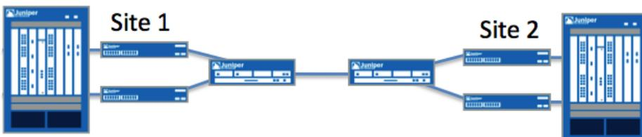
Figure 9. VPLS connected chassis cluster
