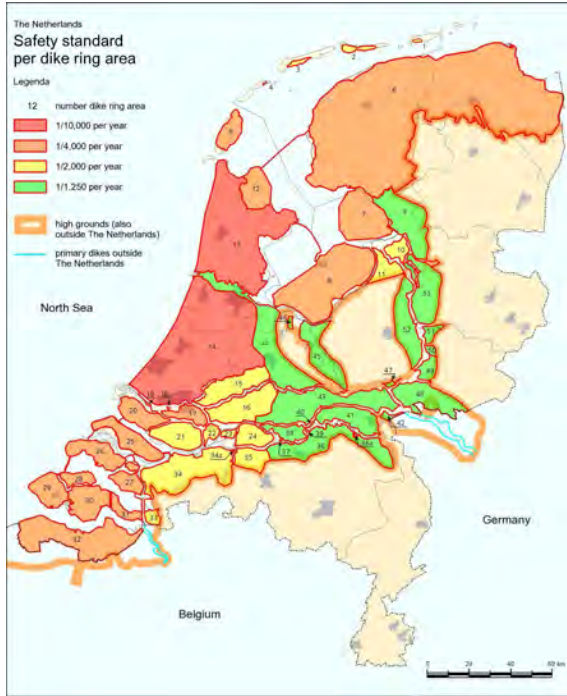
Figure 2: Dike rings in The Netherlands.
