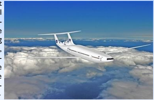
Figure 2. MIT/NASA D8.5 Advanced version of Double Bubble Aircraft Concept [Grietzner 2010; Bonnefoy 2011]
