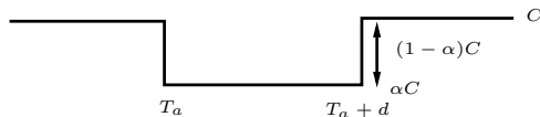
Figure: Depiction of the capacity profile under a weather-front based uncertainty set for a single affected airspace element.
