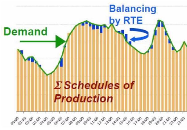
**Figure 3.** Scheduling the generation units to cover the anticipated demand is usually made day-ahead. Dispatch can be fine-tuned closer to real time. During the operating hour, balancing (operating reserves) are used to maintain the balance — load following by manual dispatch and automatic regulation in some power plants to follow the second to minute variability. (Source: RTE, the transmission system operator of France).
