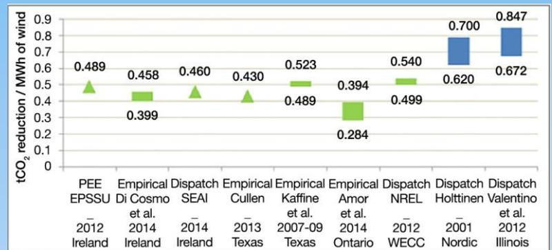
Figure 1. Examples of wind power impact on emission reductions, as g of CO<sub>2</sub> per kWh wind power generated. The green ones are from power systems where wind power replaced mostly gas-fired generation and the blue ones where mostly coal-fired generation is replaced (Source: Holttinen et al., 2014)
