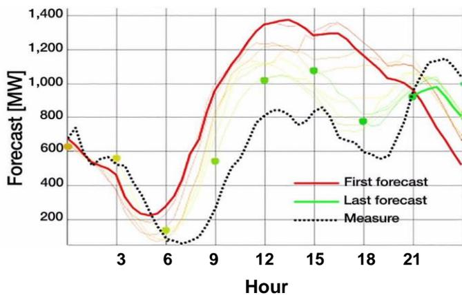
**Figure 2.** Short term forecasting of wind power generation, example showing how forecast accuracy improves with shorter forecast horizon. The first forecast 24 to 48 hours ahead in red, last forecast 6 to 30 hours ahead in green and measured power in black. (Source: Hydro Quebec)
