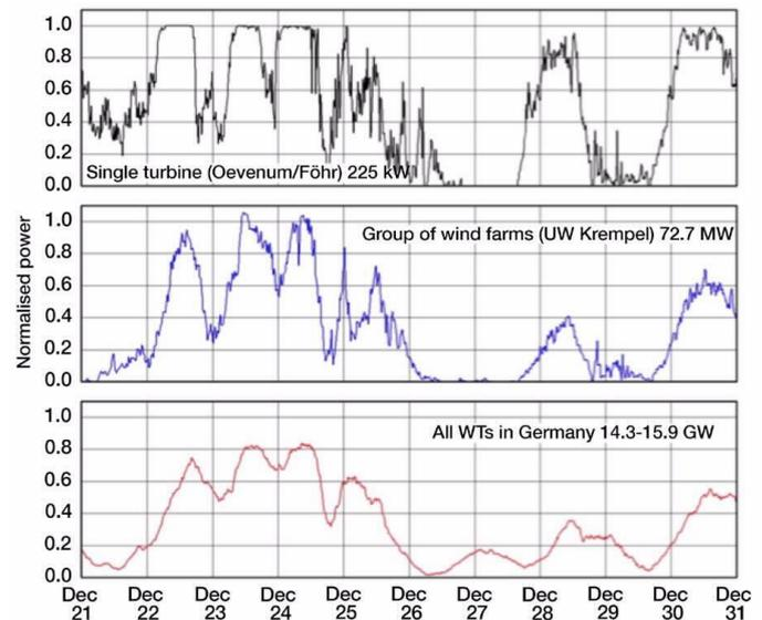
**Figure 1.** Aggregated generation from multiple wind power plants is a smoother curve than that of a single turbine. The minute and hour changes are smaller, and also the range will be reduced, not reaching full installed power from all turbines simultaneously. As seen in the middle plot, the generation of wind power from a small area can sometimes exceed the installed capacity. (Source: Task 25 summary report, 2009)
