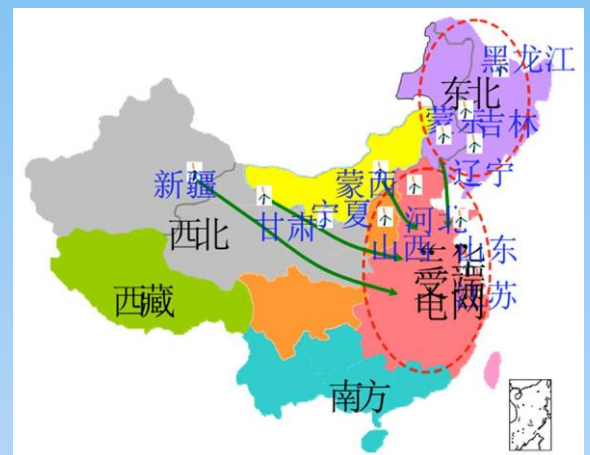
Figure 1. Example of wind power buildout from China that requires new transmission links. Large wind power plants are planned in the Northern part of China where there is not much consumption. Extra high voltage transmission lines are planned to transfer the power to load centres. (Source: SGERI)
