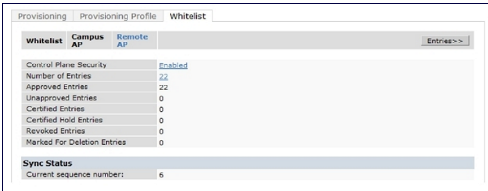
Figure 5 Control Plane Security Settings
