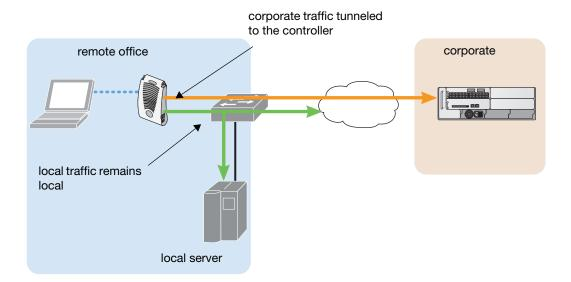
Figure 2 shows that corporate traffic is GRE tunneled to the controller through a trusted tunnel and that local traffic is source NATed and bridged on the wired interface based on the configured user role and session ACL. Split tunnel environments support both 802.1x and PSK authentication.
