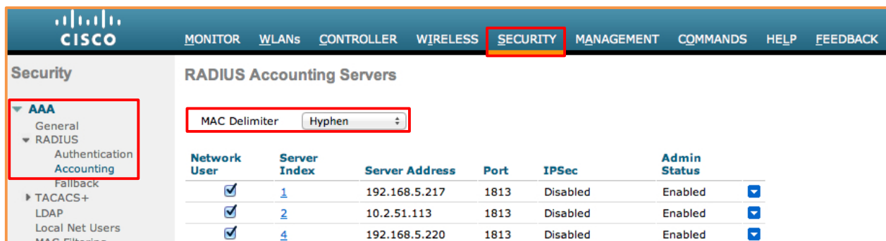
Figure 6: Configuring RADIUS accounting on Cisco WLC
