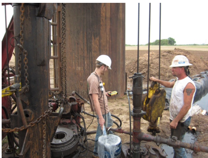
Monitoring the physical parameters of brine pumped from 5000 feet using a HACH hydrolab MS5
