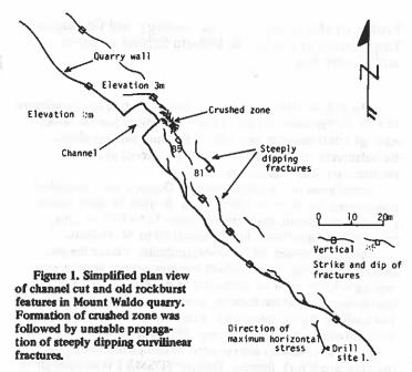
At the Mount Waldo quarry, the maximum horizontal stress direction at the south end of this zone in the uppermost sheet (which is the stratigraphically nearest measurement to the rockburst) is N19°W. The direction of the old channel is N50°E, forming an angle of approximately 70° with the maximum horizontal stress. The sheared and crushed zone direction of N28°W corresponds closely to the fracture directions of Holzhausen (1977). These features are shown in Figure 1.
