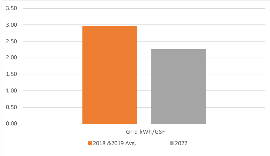
Figure 1. kWh consumed from grid per gross square foot of UMass building space
