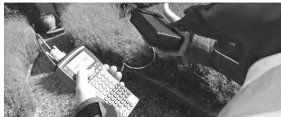
Figure 5-14. Submetering system with an RF handheld terminal.
