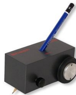
Figure 2: Apparatus used for the pencil hardness test:
