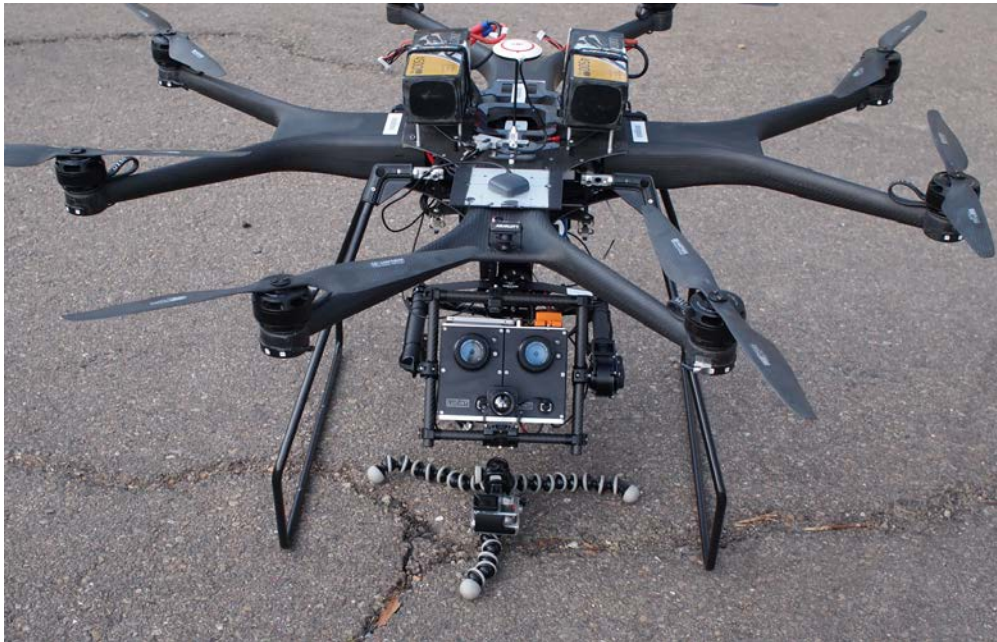
Visible + Near IR + Longwave IR Payload
