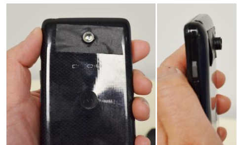
DIY microscope lens on cell phone camera
