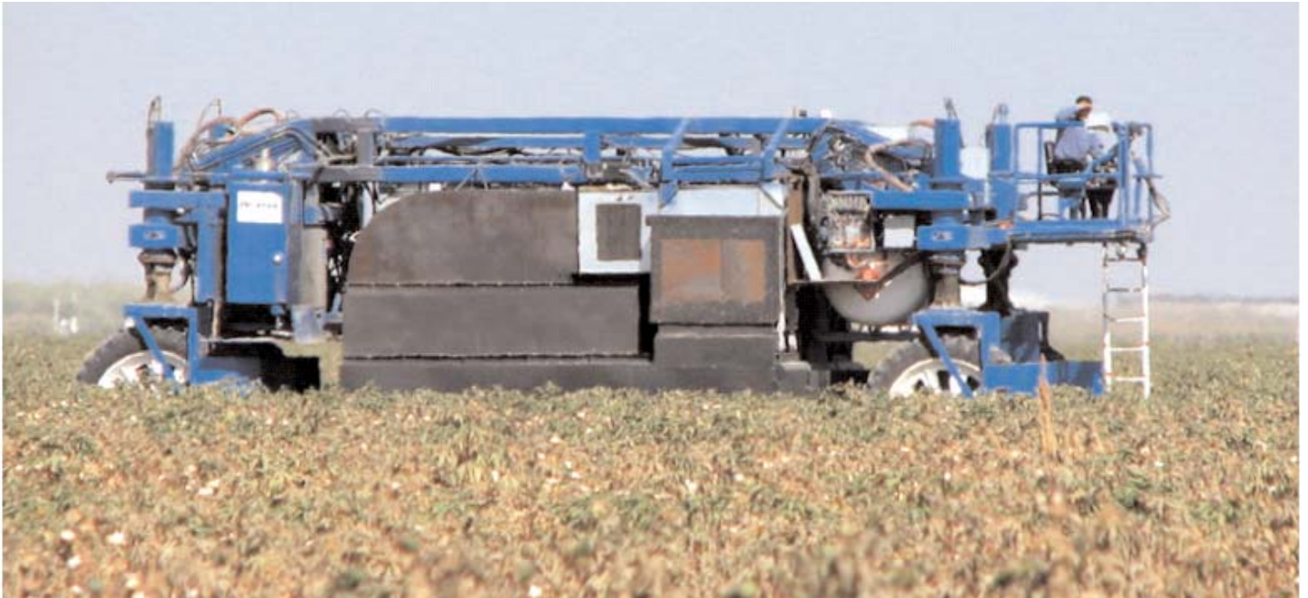
Figure 2. Commercial thermal defoliator treating organic cotton. Leaves in the foreground were treated earlier this day and were already discolored and desiccating.
