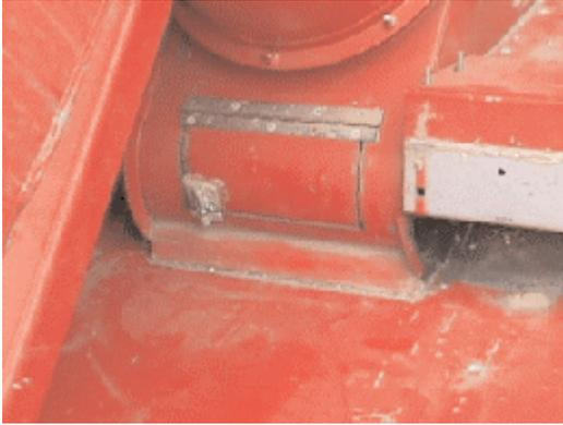
In addition, all exposed ends of sheet metal and corners should be caulked to prevent kernel lodging.
