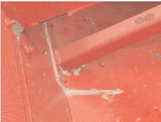
A door is added to the horizontal return auger. Note the door is taped with duct tape to seal joints.
