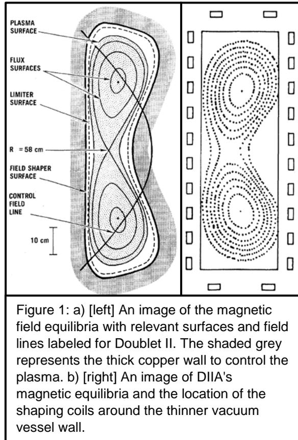
Figure 1: a) [left] An image of the magnetic field equilibria with relevant surfaces and field lines labeled for Doublet II. The shaded grey represents the thick copper wall to control the plasma. b) [right] An image of DIIA's magnetic equilibria and the location of the shaping coils around the thinner vacuum vessel wall.
